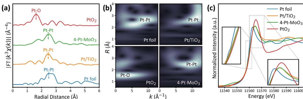
Fig. 2 (a) Fourier-transformed  $k^3$ -weighted Pt L<sub>3</sub>-edge EXAFS spectra in *R*-space, (b) corresponding WT-EXAFS contour plots, and (c) normalized XANES spectra of the PtO<sub>2</sub>, Pt foil, Pt/TiO<sub>2</sub> and 4-Pt–MoO<sub>3</sub> catalysts.
