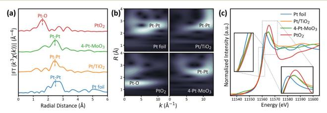
Fig. 2 (a) Fourier-transformed  $k^3$ -weighted Pt L<sub>3</sub>-edge EXAFS spectra in *R*-space, (b) corresponding WT-EXAFS contour plots, and (c) normalized XANES spectra of the PtO<sub>2</sub>, Pt foil, Pt/TiO<sub>2</sub> and 4-Pt-MoO<sub>3</sub> catalysts.
