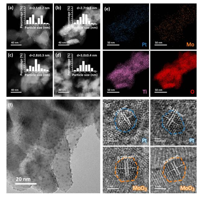
Fig. 1 HAADF-STEM images and corresponding particle size distributions of the (a) 6-Pt-MoO<sub>3</sub>, (b) 4-Pt-MoO<sub>3</sub>, (c) 2-Pt-MoO<sub>3</sub> and (d) 1-Pt-MoO<sub>3</sub> catalysts. (e) HAADF-STEM EDS mapping images, (f) TEM image and (g) HRTEM images of the 4-Pt-MoO<sub>3</sub> catalyst.
