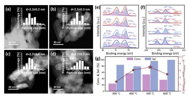
Fig. 5 HAADF-STEM images and corresponding particle size distributions of  $4-Pt-MoO_3$  reduced at (a) 300, (b) 400, (c) 500 and (d) 600 °C. (e) Pt 4f and (f) Mo 3d XPS spectra of  $4-Pt-MoO_3$  catalysts reduced at various temperatures. (g) Catalytic performance of  $4-Pt-MoO_3$  catalysts reduced at various temperatures.
