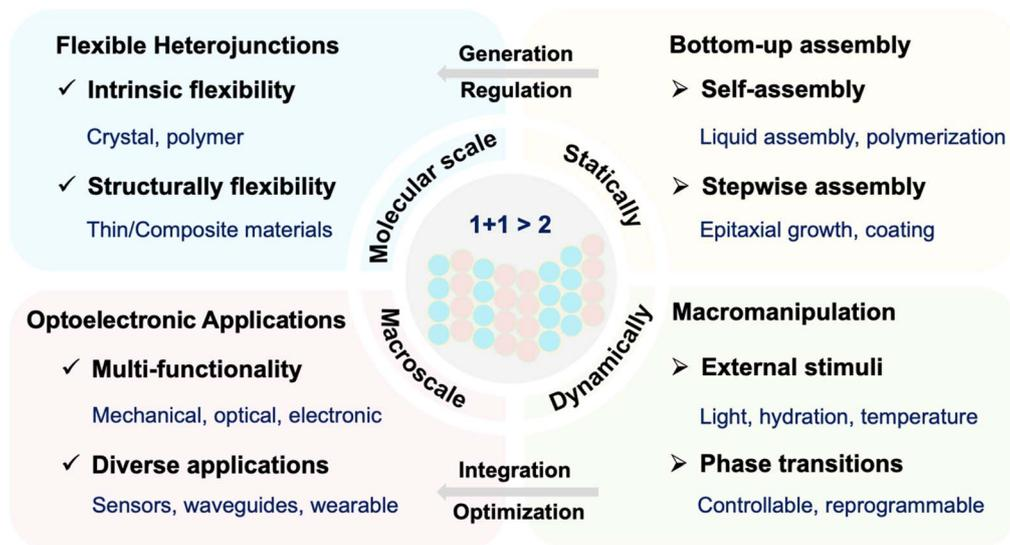
Scheme 1 Assemblies, methods and applications of flexible heterojunctions.
