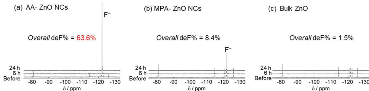
Fig. 2  $^{19}\text{F}$ -NMR spectra of the deuterated water solution containing PFOS, TEOA, and ZnO photocatalysts before and after irradiation of 365 nm light (500 mW). (a) AA-capped ZnO NCs, (b) MPA-capped ZnO NCs, and (c) bulk ZnO were used as photocatalysts.
