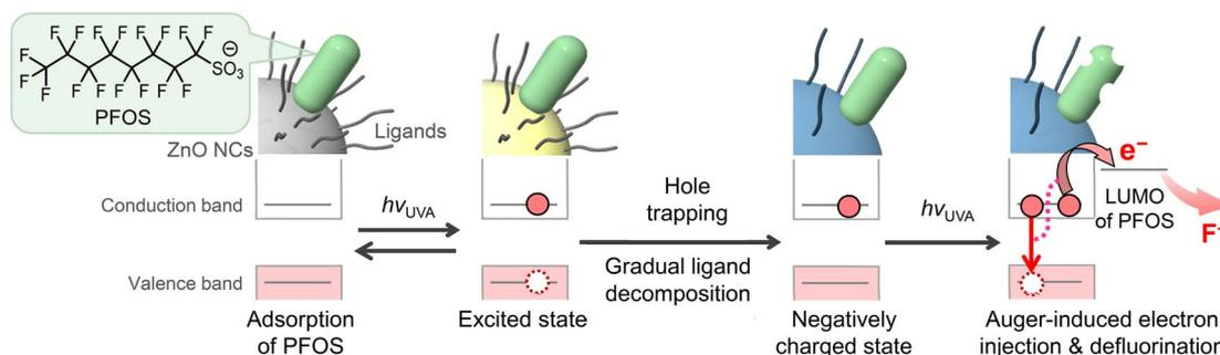
Fig. 1 Photocatalytic decomposition mechanism of PFOS by ZnO NCs.  $h\nu_{UVA}$  indicates the irradiation of 365 nm light. Surface ligands are gradually replaced with TEOA and degraded products probably related to TEOA during the decomposition of PFOS and pristine ligands.
