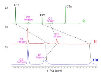
Fig. 2  $^{13}$ C NMR spectra of systems (a) 2I, (b) 1I, and (c) 1Br recorded by using MAS techniques at laboratory temperature (see the SI).
