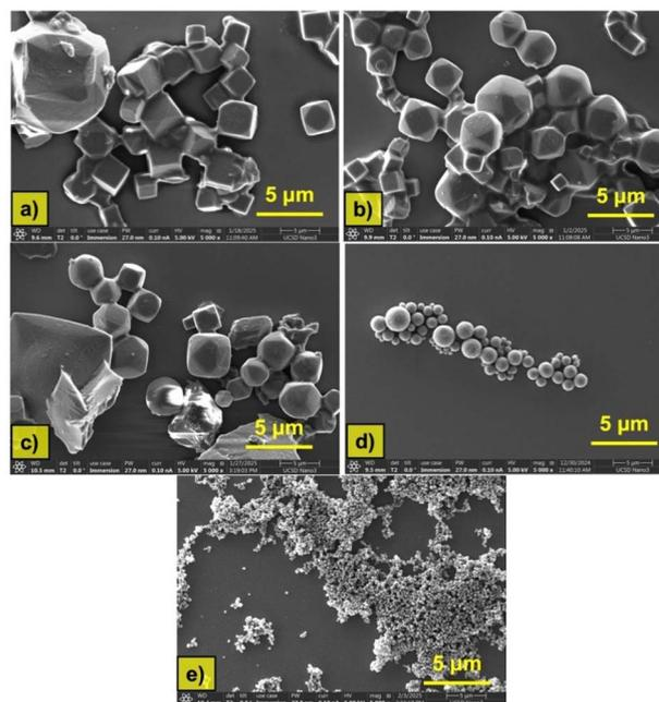
Fig. 4 SEM Images of: (a) Zn-poly(OCTbdc-5a)<sub>35</sub>, (b) Zn-*t*Bu-poly(OCTbdc-5a)<sub>29</sub>, (c) Zn-Py-poly(OCTbdc-5a)<sub>29</sub>, (d) Zn-PS<sub>12</sub>-*block*-poly(OCTbdc-5a)<sub>23</sub>-*block*-PS<sub>12</sub>, and (e) Zn-PS<sub>30</sub>-*block*-poly(OCTbdc-5a)<sub>23</sub>-*block*-PS<sub>30</sub>.
