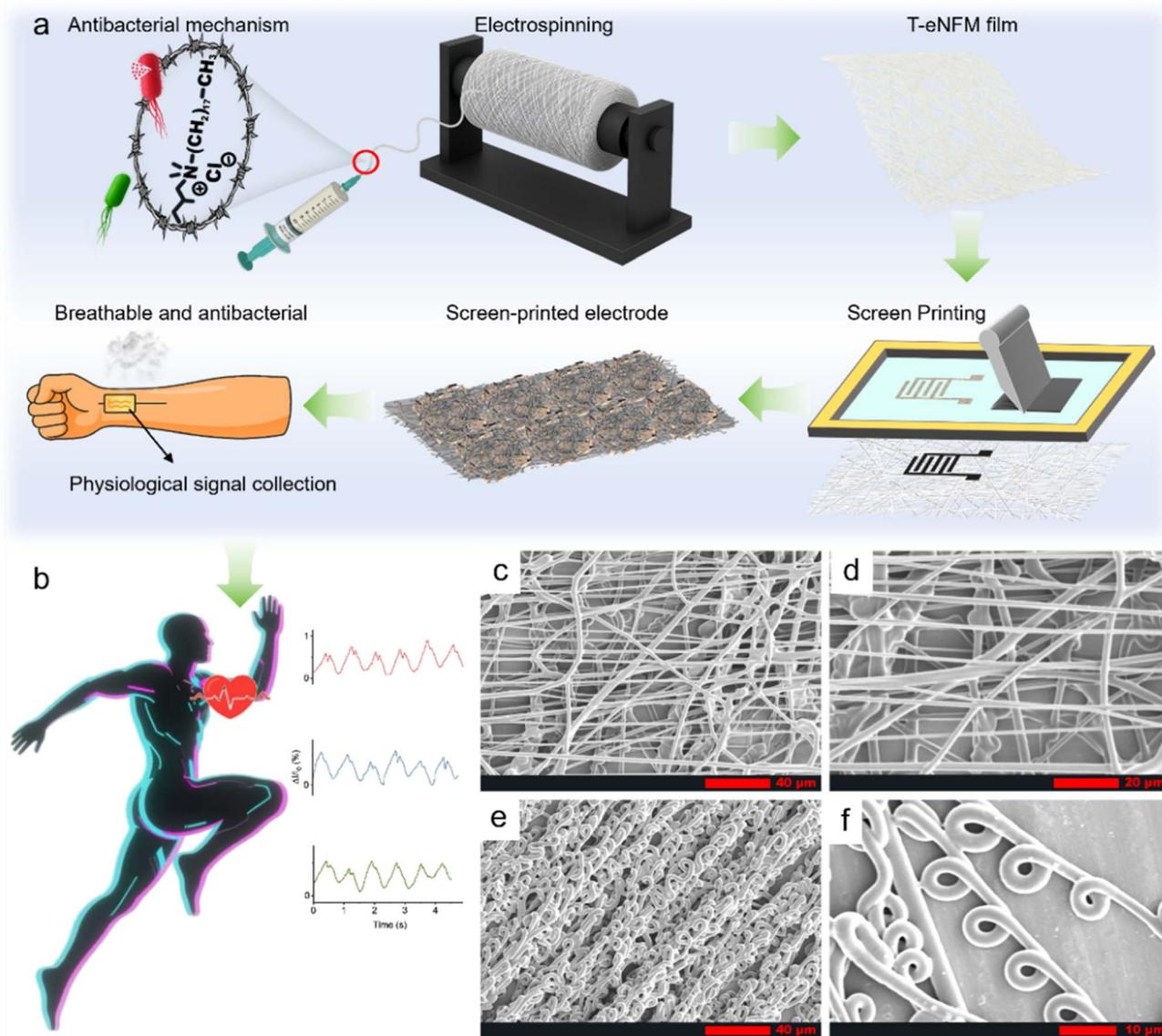
**Fig. 1** (a) Design and preparation of antibacterial and breathable electronic skin. (b) Electronic skin can be applied to human body sensing and for detecting physiological signals of the cardiovascular system. SEM images of the (c and d) fiber structures of T-eNFM-0 and (e and f) the regular spiral fiber structure presented by T-eNFM-3 at different magnifications.
