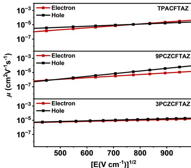
Fig. 3 Carrier mobility curves of TPACFTA Z, 9PCZCFTA Z and 3PCZCFTA Z.
