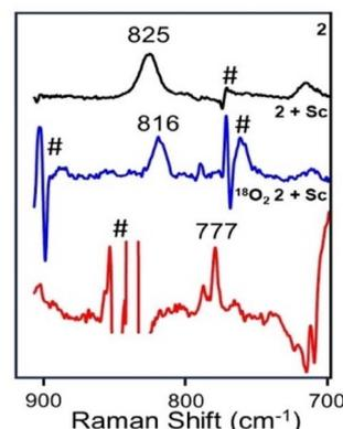
Fig. 2 Resonance Raman spectra at 77 K with  $135^\circ$  backscattering of **2** (561 nm excitation) and **2+Sc** (457 nm excitation). Black:  $0.5\text{ mM}$   $^{16}\text{O}_2\text{-2}$  in MeCN; Blue:  $0.5\text{ mM}$   $^{16}\text{O}_2\text{-2+Sc}$  in MeCN; Red:  $0.5\text{ mM}$   $^{18}\text{O}_2\text{-2+Sc}$  in  $\text{CD}_3\text{CN}$ . # indicates artifacts from solvent subtraction.
