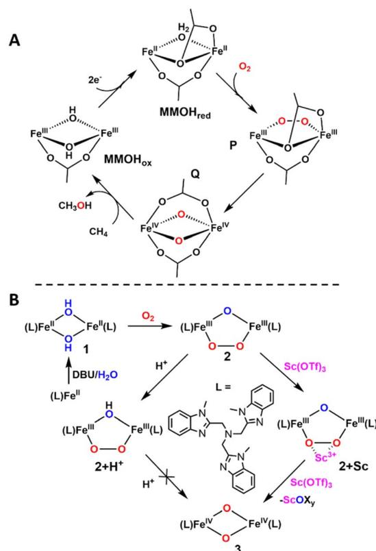
Scheme 1 (A) Proposed catalytic cycle of sMMO and (B) generation of intermediates 2, 2+H<sup>+</sup>, 2+Sc, and 3 in the biomimetic system.
