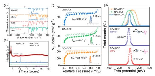
Fig. 2 Structural characterization of QiCOFs. (a) FT-IR spectra of QZwiCOF. (b) Experimental and simulated XRD patterns of QZwiCOF. (c)  $N_2$  adsorption—desorption isotherms, with pore size distributions calculated by the NLDFT method for QiCOFs. (d) Mean zeta potential of QiCOFs dispersed in ethanol and mean zeta potential of QZwiCOF under varying pH conditions.
