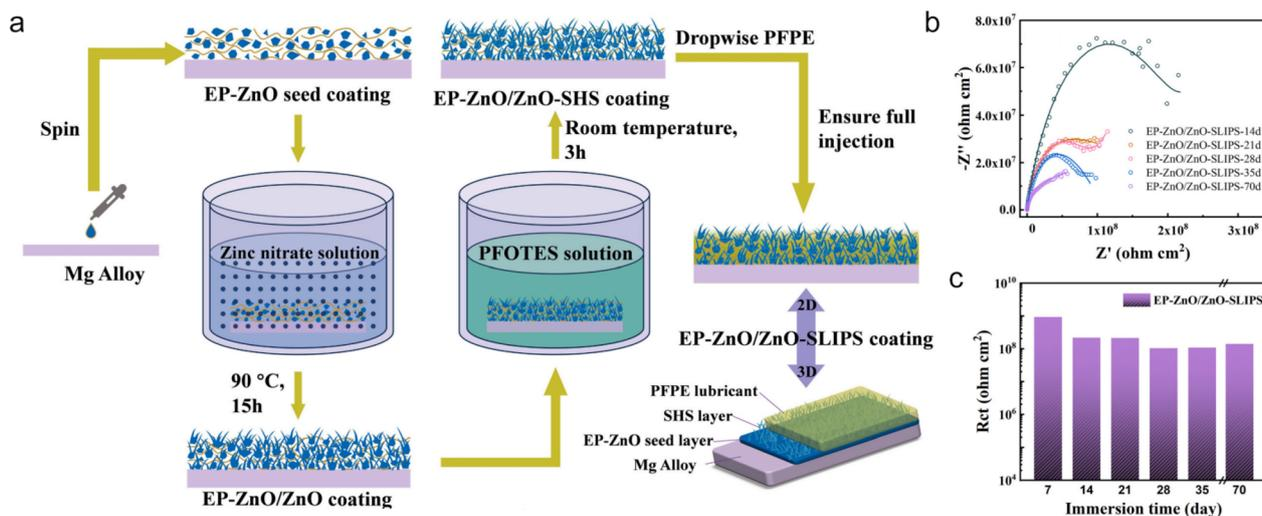
Fig. 6 (a) Preparation of EP-ZnO/ZnO-SHS and EP-ZnO/ZnO-SLIPS coatings. (b) EIS plots of EP-ZnO/ZnO-SLIPS coatings. (c)  $R_{ct}$  change of EP-ZnO/ZnO-SLIPS coatings. Adapted with permission from ref. 62. Copyright 2024 Elsevier.
