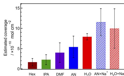
Fig. 4 Estimated coverages from the SERS intensity after 60 s illumination are shown as brown, green, purple, blue, and red color bars for Hex, IPA, DMF, AN, and  $\text{H}_2\text{O}$ , respectively. In the 100 mM  $\text{NaClO}_4$  solution  $\text{H}_2\text{O}$  (blue) and AN (red) are shown as shaded bars. Black lines correspond to deviations of those estimated coverages.
