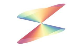
Fig. 9 Schematic illustration of a conical intersection for a twodimensional system. The seam of the conical intersection consists of only one point. This point separates two adiabatic states from each other while the colors represent diabatic characters.
