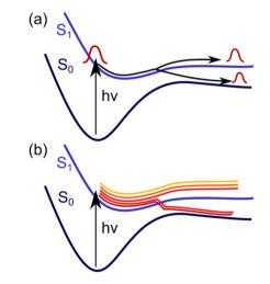
Fig. 2 Quantum (a) and classical (b) propagation of the nuclei in excited-state molecular dynamics simulations. Reproduced from ref. 8 under CC-BY 4.0.
