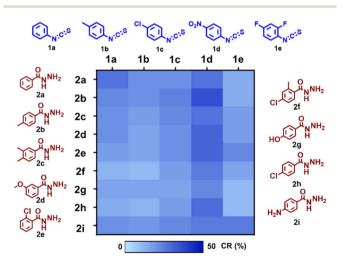
Fig. 3 Heatmap showing the cyclodesulfurization reaction outcomes using various isothiocyanates (1a–1e) and benzhydrazides (2a–2i) in methanol, with manual preparation of reaction mixtures and analysis by nESI (distance was kept at 1 cm and total concentration 5 mM). The heatmap is based on conversion ratios (CR) calculated from uncorrected ion intensities.
