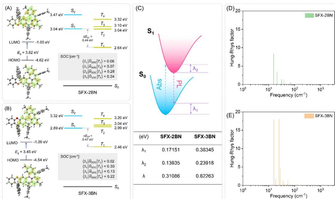
Fig. 3 The calculated FMO distribution, excited energy levels, SOC values (A and B), reorganization energy ( $\lambda$ ) (C), and Huang–Rhys (HR) factor (D and E) for the  $S_1 \rightarrow S_0$  transition of SFX-2BN and SFX-3BN, respectively.
