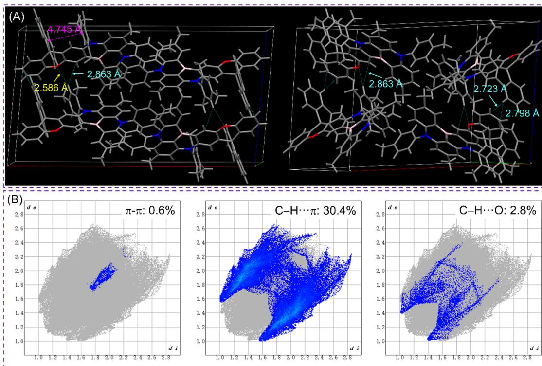
Fig. 2 (A) Packing patterns characterized by abundant C-H $\cdots$  $\pi$  and C-H $\cdots$ O bonds and (B) the primary intermolecular interactions along with their respective proportions in the SFX-3BN crystal.
