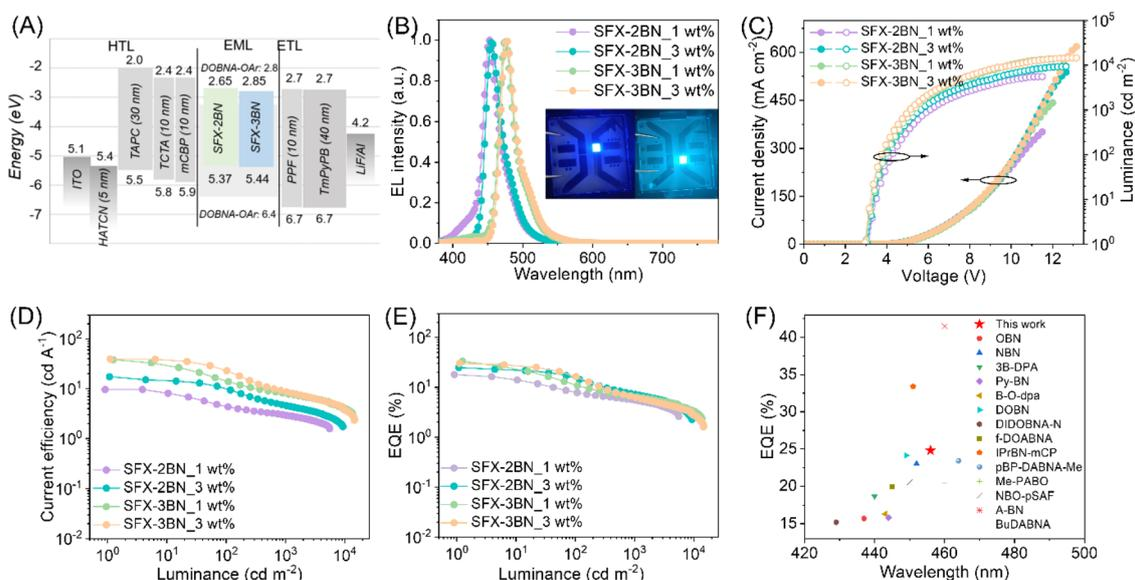
Fig. 5 (A) Schematic diagram of the device configuration, (B) the EL spectra, (C)  $J$ - $V$ - $L$  characteristics, (D and E) the efficiency curves of devices A-D, and (F) EQE versus wavelength of some representative blue OLEDs reported in the literature with CIE<sub>y</sub> ≤ 0.1.
