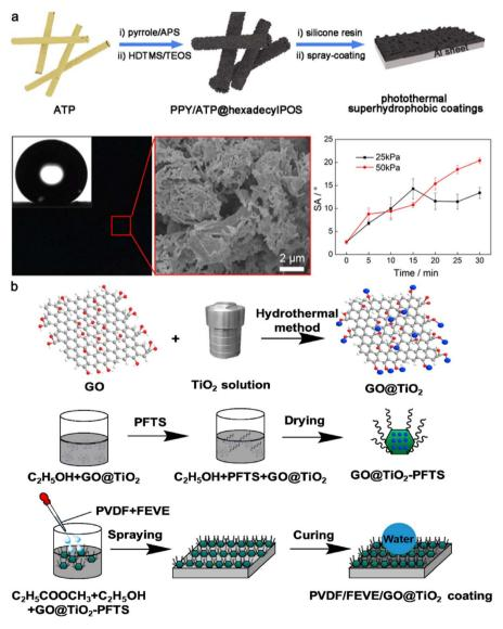
Fig. 7 (a) Schematic illustration, photographs, and mechanical robustness of the mechanically robust superhydrophobic coatings based on silicone resin. (b) Schematic illustration of the preparation of mechanically robust superhydrophobic coatings based on a fluorosilicone resin. (a) Reproduced with permission from ref. 69. Copyright 2022, Elsevier. (b) Reproduced with permission from ref. 119. Copyright 2021, Elsevier.
