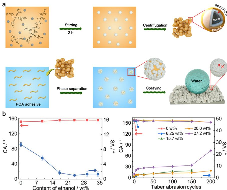
Fig. 13 (a) Schematic illustration of the superhydrophobic coatings prepared by blending adhesive microspheres with nanoparticles. (b) Effects of phase separation degree on superhydrophobicity and mechanical robustness of the superhydrophobic coatings prepared by blending adhesive microspheres with nanoparticles. (a) Reproduced with permission from ref. 64 Copyright 2023, Springer Nature. (b) Reproduced with permission from ref. 177. Copyright 2024, WILEY-VCH.
