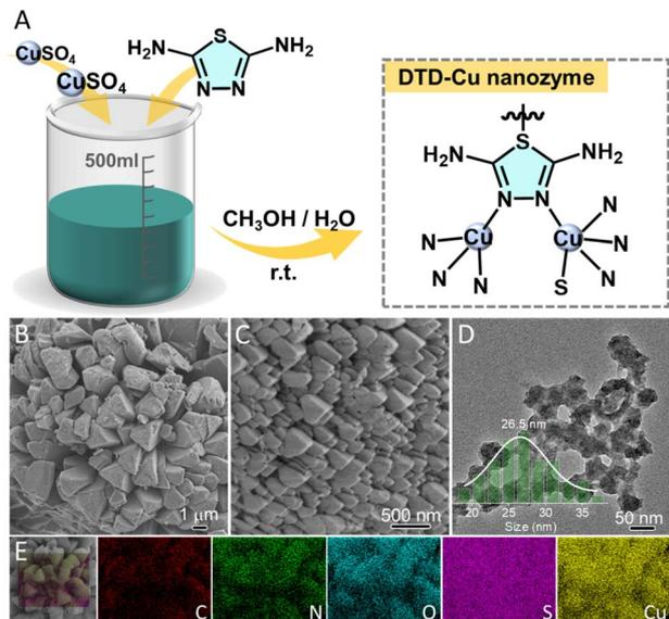
Fig. 1 (A) Schematic illustration of synthesis of the DTD-Cu nanozyme; SEM images of DTD-Cu prepared with (B) and without (C) PVP addition; (D) TEM image of DTD-Cu; (E) EDS mapping of DTD-Cu.
