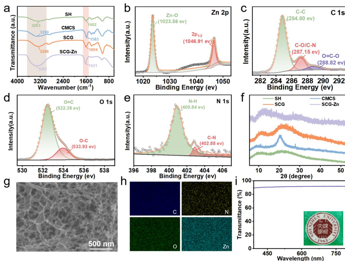
Fig. 2 (a) FTIR spectra of SH, CMCS, SCG and SCG-Zn. (b–e) XPS spectra of the Zn 2p, C 1s, O 1s and N 1s of the SCG-Zn hydrogel. (f) XRD spectra of SH, CMCS, SCG and SCG-Zn. (g) Cross-sectional SEM image and (h) elemental distribution of SCG-Zn. (i) UV-vis transmittance spectrum of SCG-Zn (inset showing its optical photograph).
