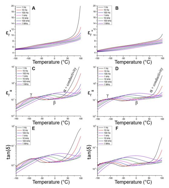
Fig. 4 Isochronal representations of  $\varepsilon_r'$ ,  $\varepsilon_r''$  and  $\tan(\delta)$  for  $\text{poly}(\text{SO}_2\text{MA-co-ANMA})$ -based SCNPs (A, C and E) and poly(CNMA-co-ANMA)-based SCNPs (B, D and F) enabling the evaluation, at fixed frequencies, of the polarization ability, dipolar relaxation behavior, and dissipative character of these materials as a function of temperature.
