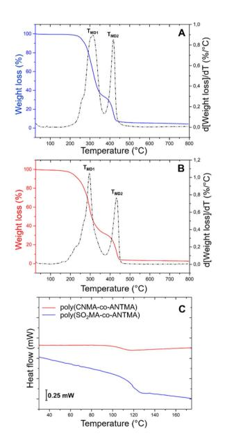
Fig. 1 TGA and DTGA thermograms of poly(SO₂MA-co-ANMA) (A) and poly(CNMA-co-ANMA) (B) linear precursors. DSC traces recorded from last heating cycles (C).
