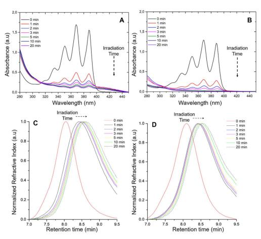
Fig. 3 UV-Vis spectra (top) and SEC traces (bottom) recorded for poly(SO<sub>2</sub>MA-co-ANMA) (A and C) and poly(CNMA-co-ANMA) (B and D) solutions after photo-irradiation for different times (see text for details).
