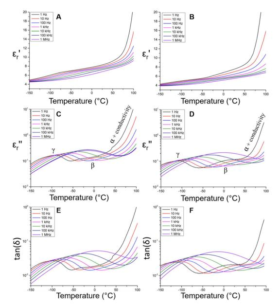
Fig. 2 Isochronal representations of and  $\tan(\delta)$  for  $poly(SO_2MA-co-ANMA)$  (A, C and E) and poly(CNMA-co-ANMA) (B, D and F) linear precursors, enabling the evaluation, at fixed frequencies, of the polarization ability, dipolar relaxation behavior, and dissipative character of the materials as a function of temperature.
