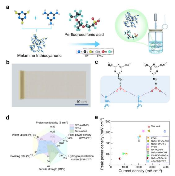
Fig. 1 PEM preparation process, proton conduction mechanism, and performance comparison. (a) Flowchart of the composite proton exchange membrane slurry fabrication process. (b) Digital photograph of large-scale composite PEMs. (c) Schematic diagram of the formation of additional hydrogen bonds between PTR and hydrated PFSA, and the proton conduction mechanism. (d) A parameter comparison radar chart. (e) Comparative data of different PEMs in related literature studies.
