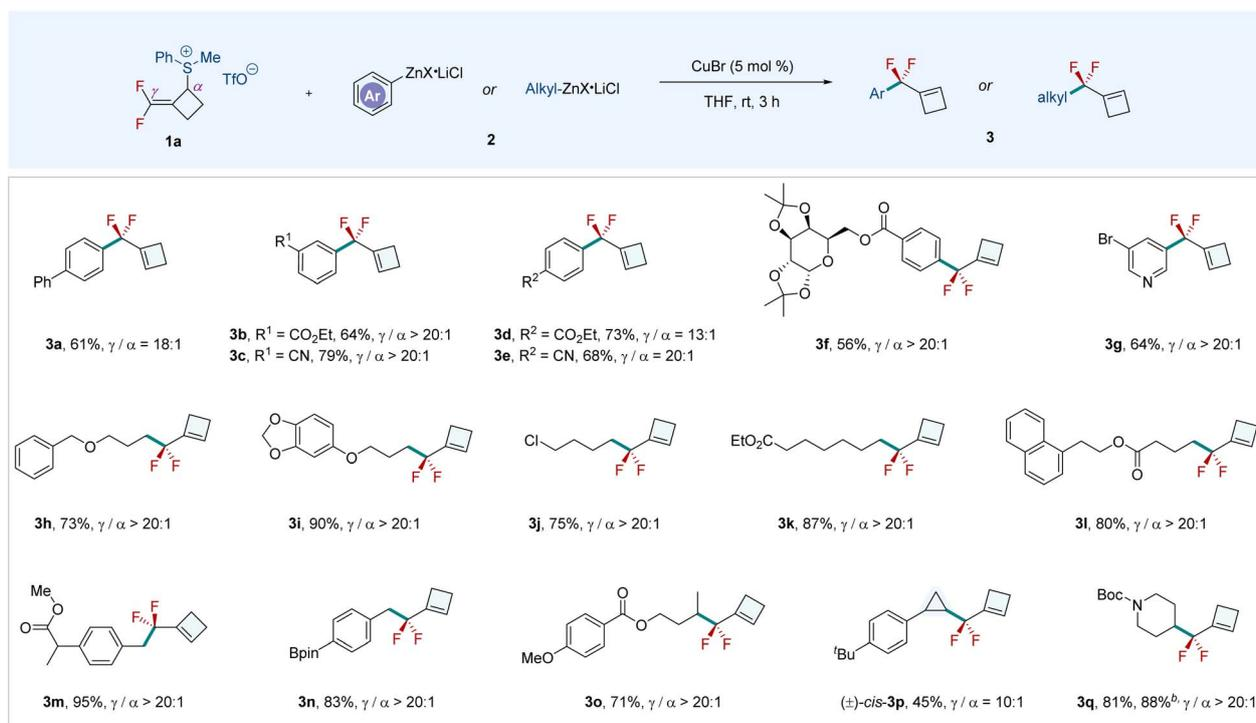
**Scheme 3** Copper-catalyzed cross-coupling of organozinc reagents with CB-DFAS **1a**. [a] Reaction conditions (unless otherwise specified): **1a** (1.05 equiv.), **2** (0.2–0.3 mmol, 1.0 equiv.), THF (2.0 mL), 3 h. All reported yields are isolated yields. [b] The reaction was conducted on a 6 mmol scale using 0.2 mol% CuBr.
