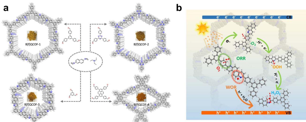
Fig. 15 (a) Synthesis of the benzo[*f*]quinoline-linked COFs *via* one-pot three-component [4 + 2] cyclic condensation. (b) The proposed mechanism diagram for the photocatalytic synthesis of  $\text{H}_2\text{O}_2$  over the B[f]QCOFs *via* both ORR and WOR pathways.
