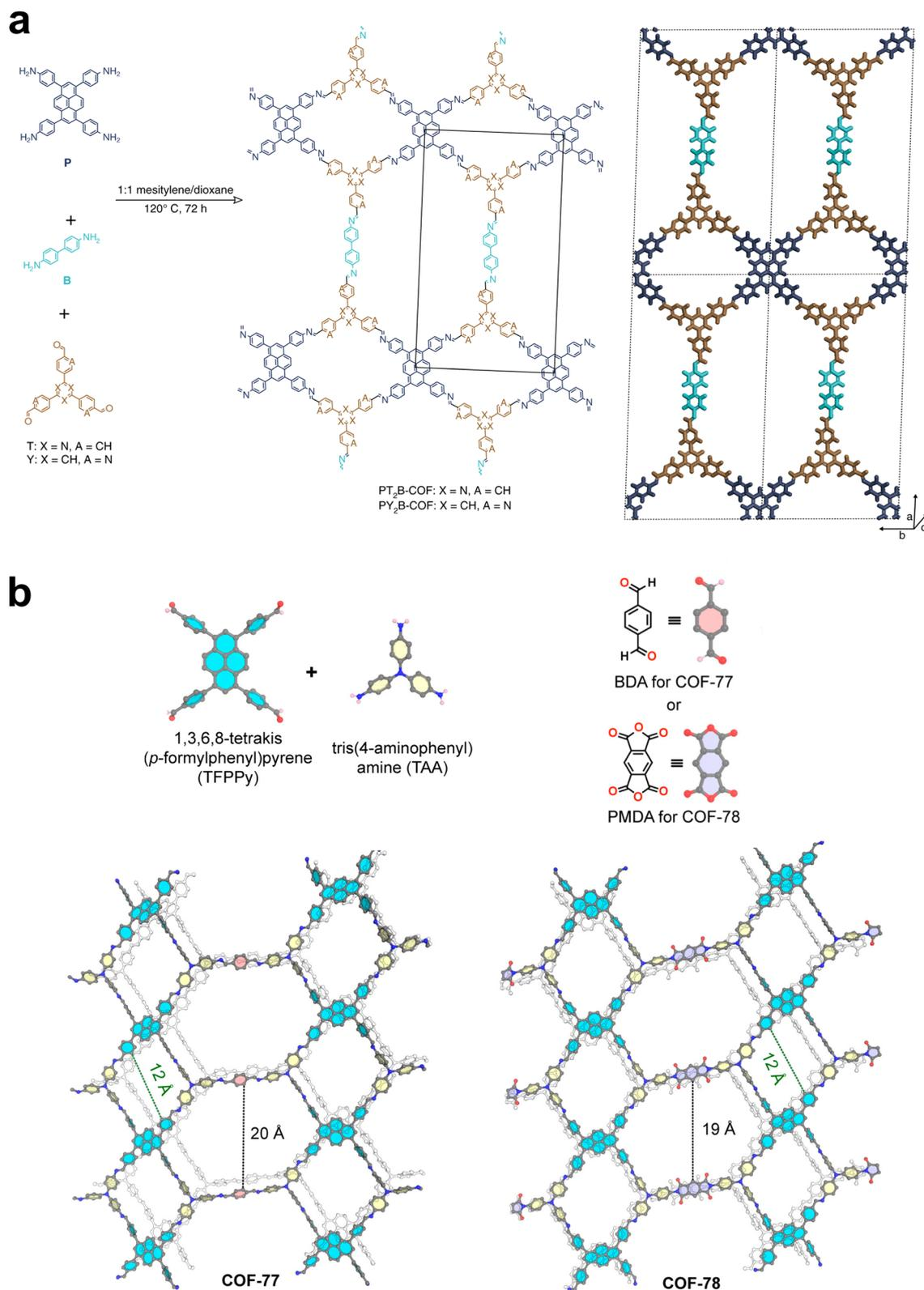
**Fig. 8** (a) Structure of PT<sub>2</sub>B-COF and PY<sub>2</sub>B-COF. (b) Synthesis of COF-76 and COF-78. Atom sphere colors: C, gray; N, blue; O, red. Hydrogen atoms, except for aldehyde- and amine-hydrogens, omitted for clarity; reproduced from ref. 59. Copyright 2020, The American Chemical Society.
