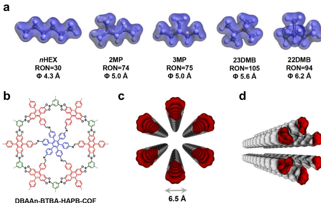
Fig. 18 (a) Hexane isomers (*n*HEX, 2MP, 3MP, 23DMB, and 22DMB) with their RONs and  $\Phi$  values. Structural formula of (b) DBAAn-BTBA-HAPB-COF. (c) Top-view and (d) side-view van der Waals surfaces associated with the 1D channels running through DBAAn-BTBA-HAPB-COF.
