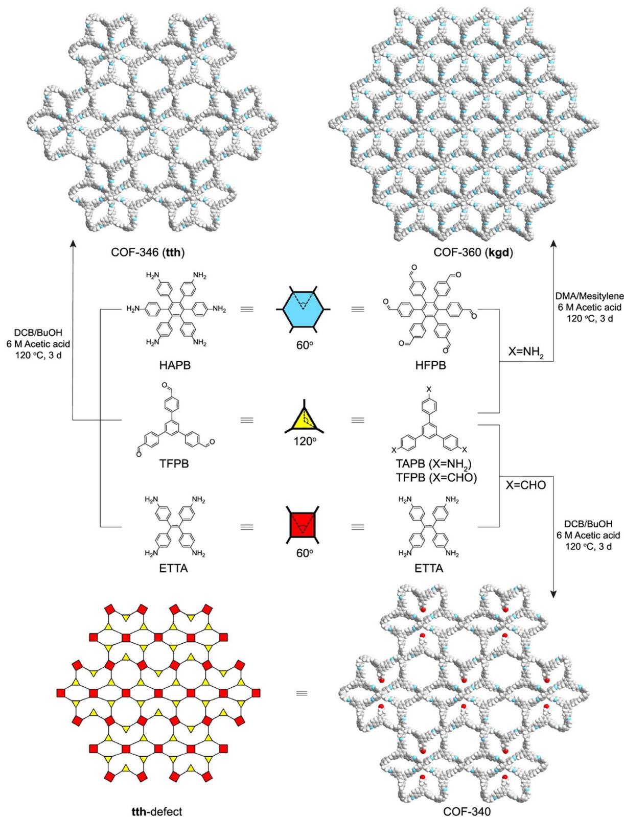
Fig. 7 Synthetic scheme for COF-346, -340, and -360. Color code: H, white; C, gray; N, blue; O, red. Frustrated aldehydes are randomly oriented in the COF-340 structure; reproduced from ref. 28. Copyright 2019, The American Chemical Society.
