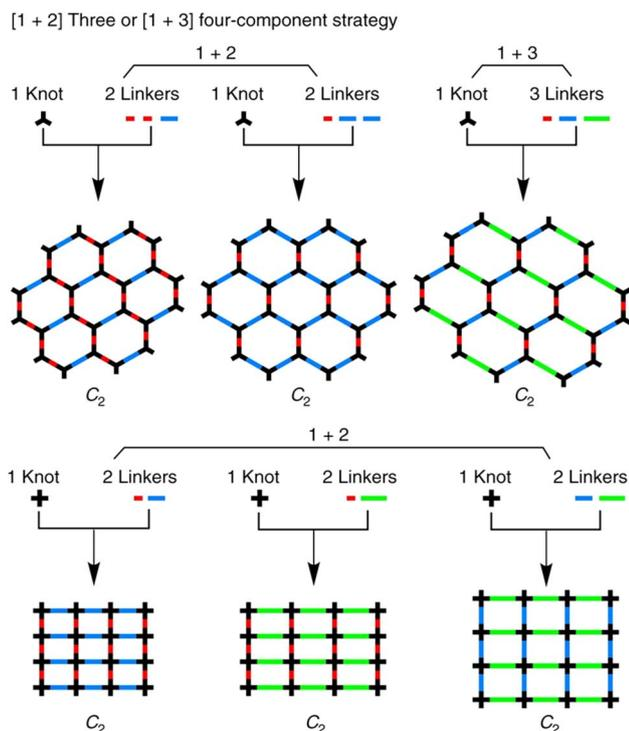
Fig. 6 Multiple-component  $[1 + 3]$  or  $[1 + 4]$  strategy for the synthesis of hexagonal and tetragonal MC-COFs. Three linkers shown in different colors and with different lengths are used to illustrate the typical knot-linker combinations in the MC strategy.
