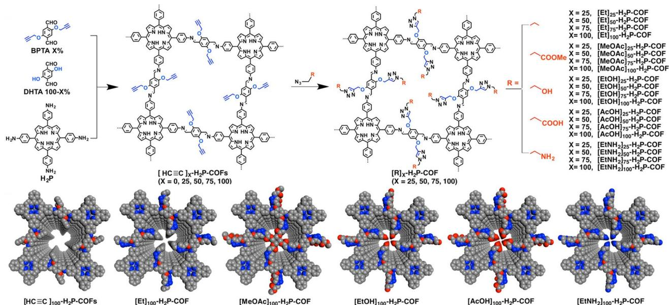
Fig. 4 Schematic of pore surface engineering of imine-linked COFs with various functional groups via click reactions and pore structures of COFs with different functional groups (Gray, C; Blue, N; Red, O); reproduced from ref. 53. Copyright 2015, The American Chemical Society.
