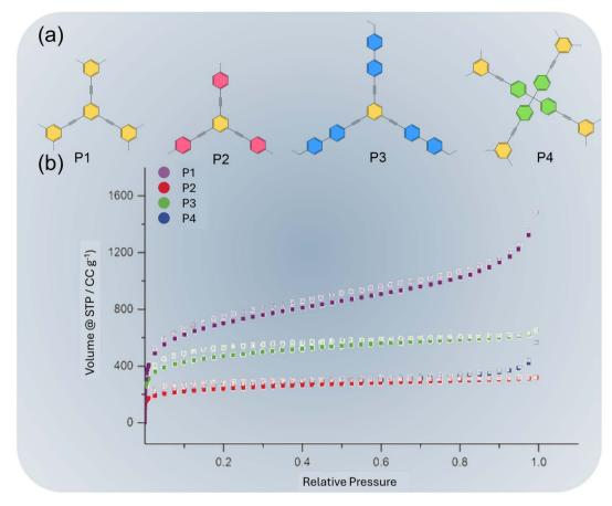
Fig. 3 (a) Copper-free CMPs synthesized from 1,3,5-triethynylbenzene and used as supercapacitor electrodes and (b) corresponding  $N_2$ adsorption-desorption isotherms.74 Adapted with authorization of Wiley
