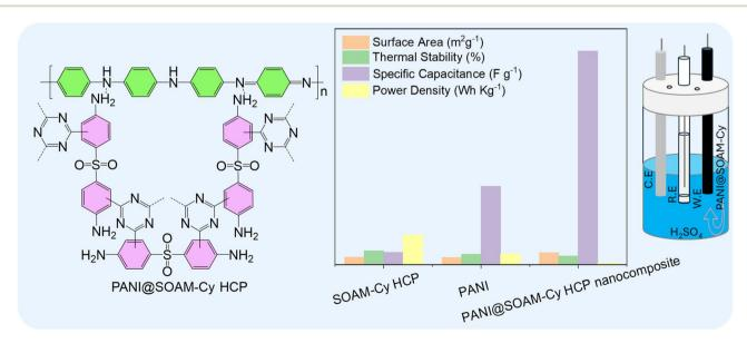
Fig. 22 Molecular structure of the PANI@SOAM-Cy HCP and the influence of polyaniline (PANI) integration on the physical and electrochemical properties of the porous organic polymer (POP).<sup>111</sup> Adapted with authorization of Elsevier.
