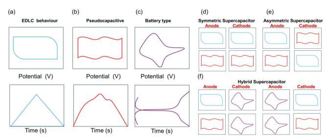
Scheme 3 Illustration of current–potential characteristics for EDLCs (a), pseudocapacitors (b), and battery-type systems (c), showing the contrast between potential-independent and potential-dependent charge storage, along with different types of supercapacitors—symmetric (d), asymmetric (e), and hybrid configurations (f).
