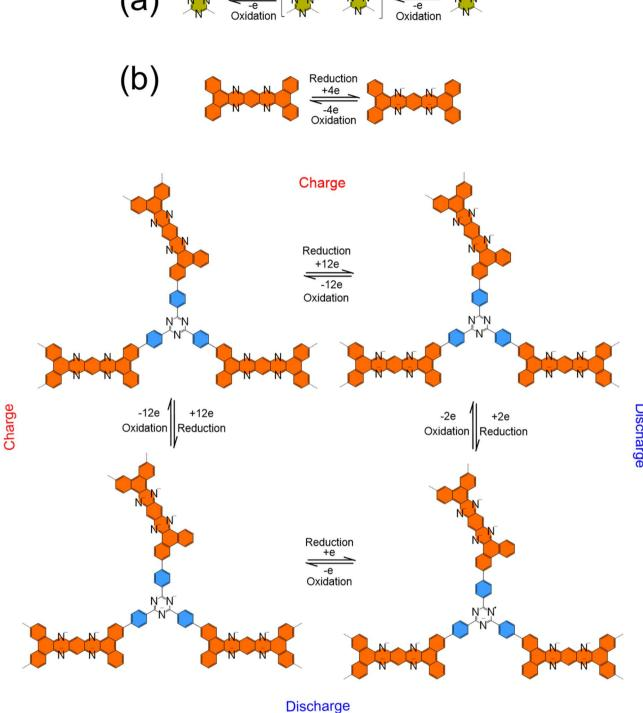
Fig. 13 (a) Schematic representation of the redox electron transfer mechanism during the charge and discharge processes occurring within nitrogen-rich cyanuric chloride units.<sup>125</sup> (b) Proposed redox pathways for QP, TPT, and the resulting TPT-QP CMP.<sup>20</sup>
