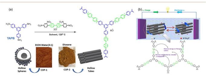
Fig. 16 (a) Schematic representation of the solvothermal synthesis of viologen-based conjugated organic polymers (COPs) through the Zincke reaction and (b) proposed charge transfer and storage mechanism occurring in COP-2 during the electrochemical charging and discharging processes.<sup>131</sup> Adapted with authorization of Elsevier.
