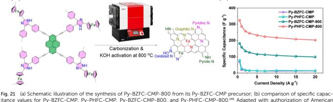
itance values for Py-BZFC-CMP, Py-PHFC-CMP, Py-BZFC-CMP-800, and Py-PHFC-CMP-800. 441 Adapted with authorization of American Chemical Society.
