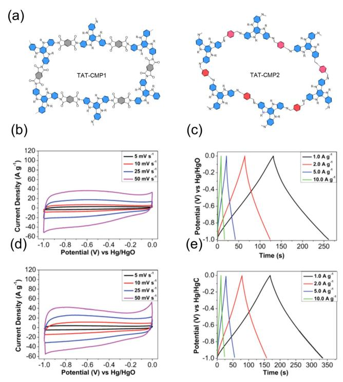
Fig. 2 (a) Schematic structures of TAT-CMP-1 and TAT-CMP-2, and (b and d) CV and (c and e) GCD analyses of TAT-CMP-1 (b and c) and TAT-CMP-2 (d and e), respectively.<sup>64</sup> Adapted with authorization of the Royal Society of Chemistry.
