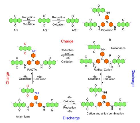
Fig. 11 Illustration of the charge-discharge mechanism and the associated redox reactions proposed for PAQTA.<sup>117</sup>
