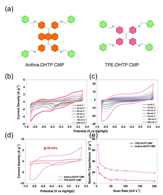
Fig. 5 (a) Chemical structures of TPE-DHTP and Anthra-DHTP CMPs, (b and c) CV analyses of TPE-DHTP and Anthra-DHTP CMPs, (d) representative CV curves of DHTP-based CMP electrodes measured at 50 mV s<sup>-1</sup>, and (e) plot illustrating the dependence of specific capacitance on the scan rate for the DHTP-CMP electrodes.<sup>80</sup> Adapted with authorization of American Chemical Society.
