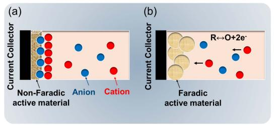
Scheme 2 Diagrammatic representations of (a) non-faradaic and (b) faradaic mechanisms of charge storage
