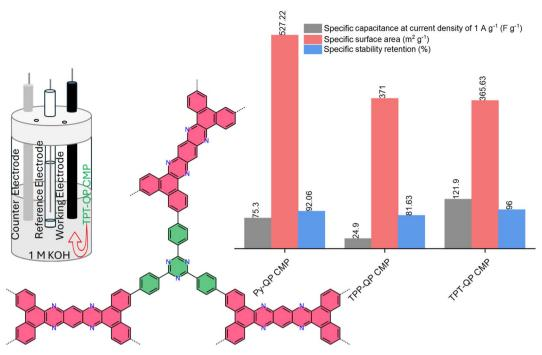
Fig. 1 Illustration showing different CMPs featuring a redox-active QP core and subunits such as Py, TPP, and TPT—with varying degrees of planarity and imine linkages—showing how these structural variations affect the physical and electrochemical properties when used as supercapacitor electrodes.<sup>20</sup> Adapted with authorization of Elsevier.
