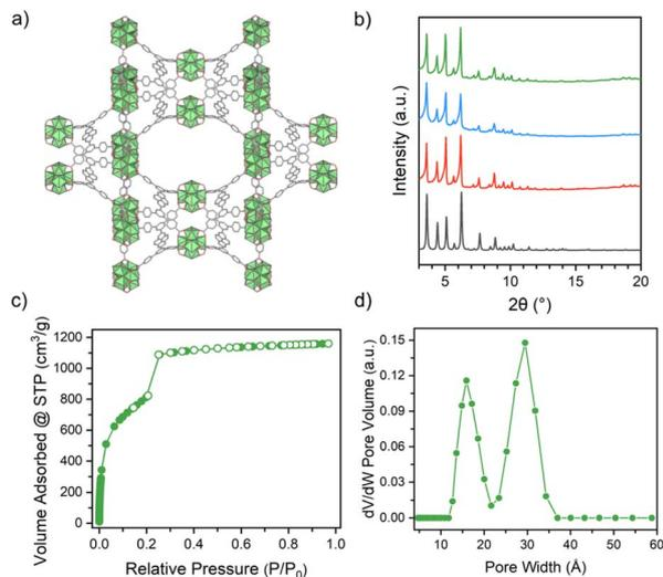
Fig. 3 (a) The structural representation of **BCN-83**; (b) PXRD patterns of simulated (black), as-made (red), acetone-exchanged (blue) and activated (green) **BCN-83**; (c)  $N_2$  sorption isotherm of **BCN-83**; (d) DFT pore size distribution of **BCN-83**.
