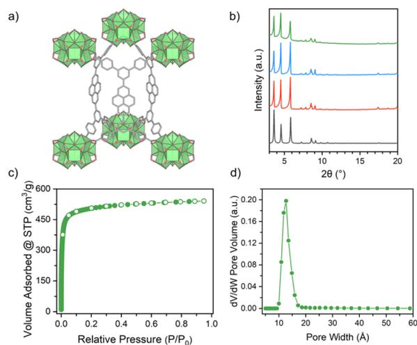
Fig. 5 (a) The structural representation of **BCN-123**; (b) PXRD patterns of simulated (black), as-made (red), acetone-exchanged (blue) and activated (green) **BCN-123**; (c)  $\text{N}_2$  sorption isotherm of **BCN-123**; (d) DFT pore size distribution of **BCN-123**.
