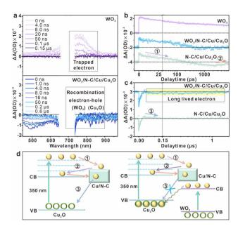
Fig. 4 (a) Transient absorption spectra of  $WO_3/N-C/Cu/Cu_2O$  and  $WO_3$ . (b and c) Kinetics of  $WO_3/N-C/Cu/Cu_2O$ ,  $N-C/Cu/Cu_2O$  and  $Cu_2O$  at 750 nm. (d) Schematic diagram of charge migration paths in  $N-C/Cu/Cu_2O$  and  $WO_3/N-C/Cu/Cu_2O$ .
