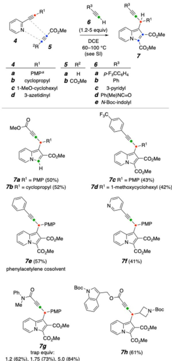
Fig. 2 Third-component trapping of free carbenes derived from alkynylpyridines **4a–d** with terminal alkynes **6a–e**. <sup>a</sup>*p*-Methoxyphenyl.
