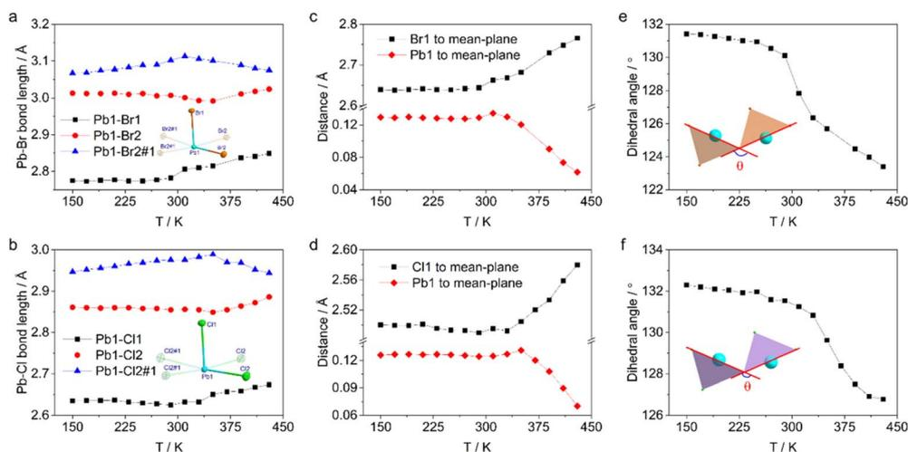
Fig. 3 Plots of Pb–X bond length vs. temperature within the range of 150–430 K for (a) PbBr<sub>5</sub> pyramid in **1** and (b) PbCl<sub>5</sub> pyramid in **2**. (c and d) Plots of distances of Pb1 and X1 (X = Br or Cl) to the basal plane of pyramids and (e and f) temperature-dependent  $\theta$  angle between the basal planes of two neighboring coordination pyramids in **1** and **2**.
