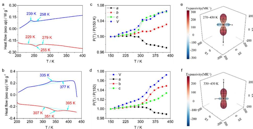
Fig. 2 DSC plots of (a) **1** and (b) **2**. Temperature dependence of relative cell parameters  $P(T)/P(150 \text{ K})$  in the  $150$ – $423 \text{ K}$  range for **1** (c) and **2** (d). 3D distribution of the direction-dependent coefficients of thermal expansion (CTE) in the HTP for **1** (e) and **2** (f).
