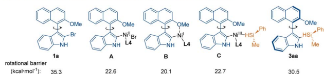
Scheme 2 Proposed reaction pathway and calculated rotational barriers.
