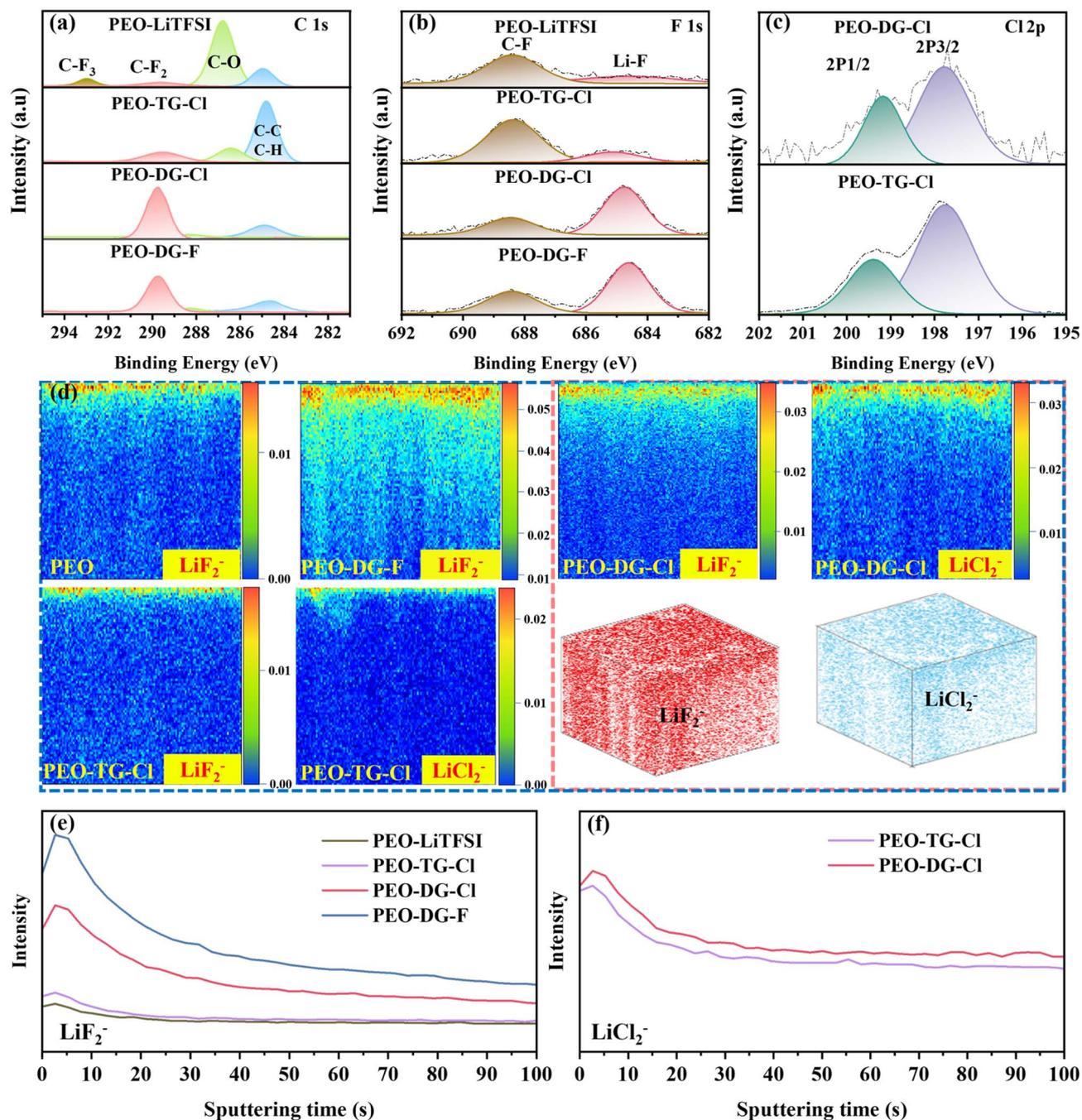
Fig. 4 CSE XPS spectra after 200 h lithium-symmetric cycling: (a) C 1s, (b) F 1s, and (c) Cl 2p. (d) Post-cycling TOF-SIMS characterization of lithium electrodes from CSE batteries.  $\text{LiF}_2^-$  content mapping and  $\text{LiF}_2^-$  signals denote LiF.  $\text{LiCl}_2^-$  content mapping and  $\text{LiCl}_2^-$  signals denote LiCl. TOF-SIMS 3D reconstruction of PEO-DG-Cl. TOF-SIMS depth profile intensity distribution (e)  $\text{LiF}_2^-$  and (f)  $\text{LiCl}_2^-$ .
