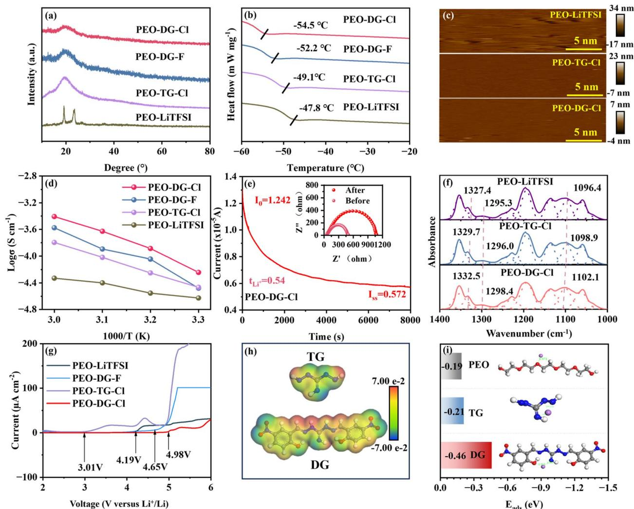
Fig. 2 (a) XRD spectra. (b) DSC curves. (c) AFM image of the CSE surface. (d) Ionic conductivity of CSEs. (e)  $\text{Li}^+$  mobility number curves of PEO-DG-Cl. (f) CSE Fourier infrared curve. (g) LSV curve. (h) TG and DG electrostatic potential distributions. (i) Binding energies of PEO chains, TG, and DG with lithium ions.
