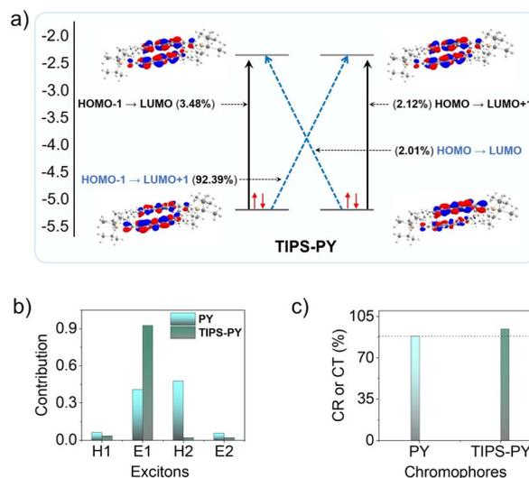
Fig. 2 (a) Illustration of the contribution of the linear combination of orbital replacement in **TIPS-PY**. (b) Plot showing comparative electron (E), and hole (H) contributions during orbital replacement in **PY** and **TIPS-PY**. (c) Percentage of charge resonance (CR) or charge transfer (CT) calculated from E and H contributions during orbital replacement in **PY** and **TIPS-PY**.
