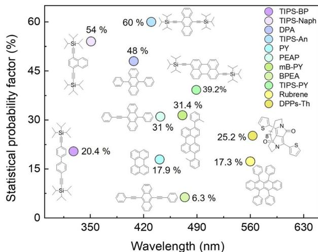
Fig. 4 Plot showing variation in statistical probability factor of various annihilators emitting across the visible spectral range. **TIPS-PY** synthesized in this work tops the list in the 470–570 nm range.
