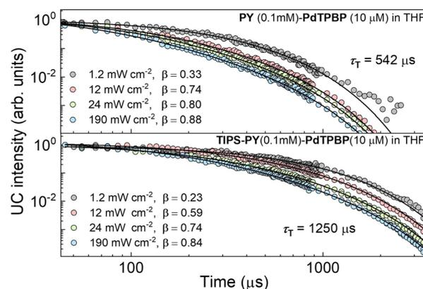
Fig. 5 Normalized UC transients of **PY** and **TIPS-PY** on a log–log scale at different excitation densities (indicated) upon sensitization with PdTPBP at 640 nm. Circles present experimental data, while solid lines show global fits with a shared  $\tau_T$ .
