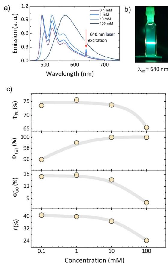
Fig. 3 (a) **TIPS-PY: PdTPBP** upconversion spectra at  $0.1$  mM,  $1$  mM,  $10$  mM, and  $100$  mM annihilator concentrations.  $640$  nm laser excitation indicated. (b) Digital image of TTA-UC emission, and (c)  $\phi_{FL}$ ,  $\phi_{TET}$ ,  $\phi_{UC}^\infty$ , and  $f$  dependence on **TIPS-PY** concentration. All solutions were prepared in deaerated THF. **PdTPBP** concentration in all UC solutions was maintained at  $0.01$  mM. The grey lines serve as a guide to the eyes.
