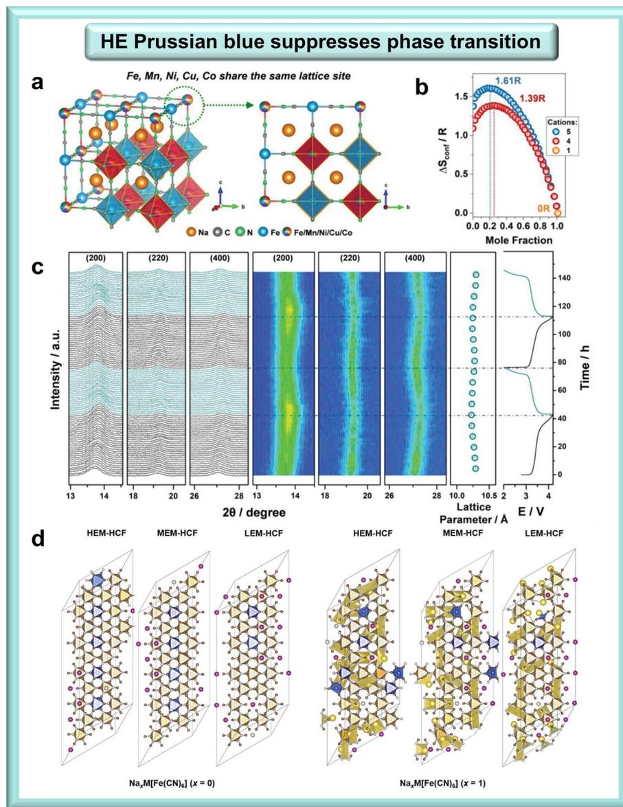
Fig. 11 (a) Schematic diagram of the crystal structure of multi-element doping. (b) *In situ* DEMS test of the HEM during the second charge/discharge. (c) *In situ* XRD patterns during charging and discharging. Reprinted with permission from ref. 95. Copyright 2021 Wiley VCH. (d) The structures of PBAs with three different entropies were simulated by using DFT calculations. Reprinted with permission from ref. 69. Copyright 2022 Wiley VCH.
