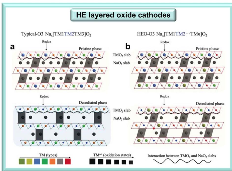
Fig. 5 (a) The conventional O3-type Na-based layered oxides contain three different TM elements. (b) The proposed HEO cathodes have multiple TM elements (TM<sub>2</sub> represents the redox elements and is marked in blue). Reprinted with permission from ref. 92. Copyright 2020 Wiley VCH.
