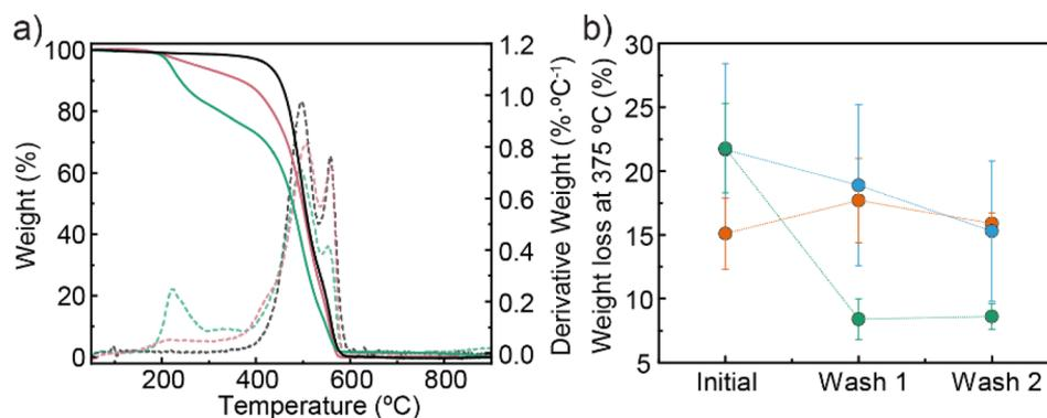
Fig. 4 (a) TGA analysis (air, 10 °C min<sup>-1</sup>) of (6,5)-SWNT (black), eW⊃SWNT (green) and the supramolecular mixture of (6,5)-SWNTs with eW (pink). (b) TGA weight losses at 375 °C (air, 10 °C min<sup>-1</sup>) before and after two hot washes in eW⊃SWNT (green), eW⊃SWNT submitted to NaBH<sub>4</sub> treatment (orange) and eR⊃SWNT (blue).
