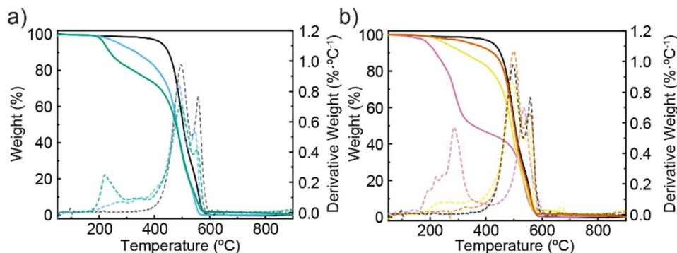
Fig. 2 (a) TGA analysis (air, 10 °C min<sup>-1</sup>) of (6,5)-SWNT (black), eW $\supset$ SWNT (green), and the mixture of 1 and 2 with (6,5)-SWNTs in the absence of cat. TFA (blue). (b) TGA analysis (air, 10 °C min<sup>-1</sup>) of (6,5)-SWNT (black), the supramolecular complexes formed by the combination of (6,5)-SWNTs and 1 (yellow) or 2 (orange) and the equimolar mixture of 1 and 2 in absence of (6,5)-SWNTs (pink).
