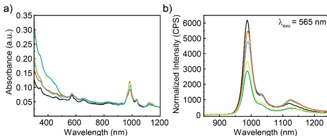
Fig. 3 (a) UV-Vis-NIR spectra (D<sub>2</sub>O (DOC, 1 wt%)) of (6,5)-SWNT (black), **eW**⊃SWNT (green), the mixture of **1** and **2** with (6,5)-SWNTs in the absence of cat. TFA (blue), the supramolecular complex formed by stirring **1** and (6,5)-SWNTs (yellow) and the supramolecular complex formed by stirring **2** and SWNTs (orange). (b) Normalized photoluminescence emission spectra with  $\lambda_{\text{exc}} = 565$  nm for the samples indicated in (a).
