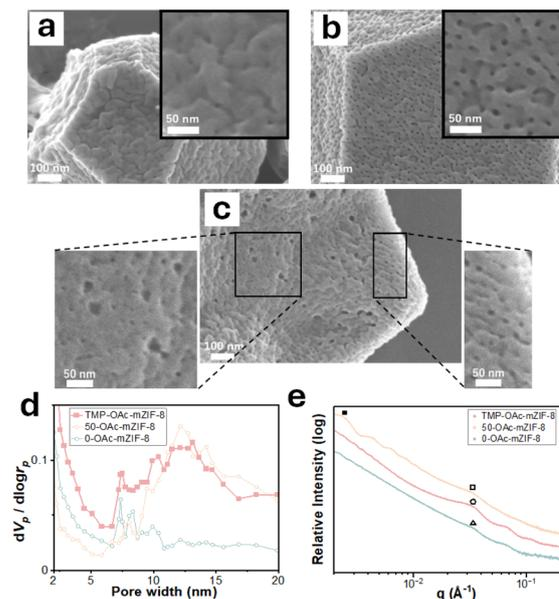
Fig. 4 SEM images of (a) 0/2 h-mZIF-8 and (b) TMP-mZIF-8. (c) Cross-sectional SEM image of TMP-mZIF-8, showing magnified views of the core and shell regions. (d) BJH pore size distributions and (e) SAXS 1D profiles of TMP-mZIF-8, 50-mZIF-8, and 0-mZIF-8.
