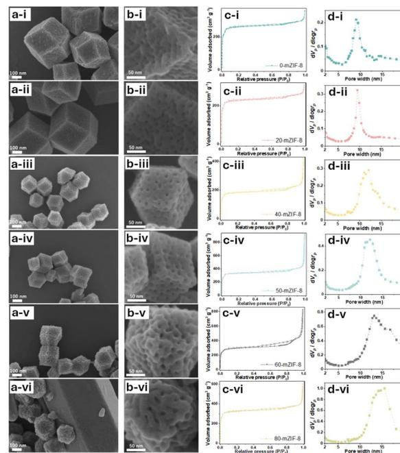
Fig. 1 (a) SEM images, (b) magnified SEM images, (c) nitrogen adsorption–desorption isotherms, and (d) BJH pore size distributions of *X*-mZIF-8, where *X* represents the synthesis temperature (°C): (i) 0 °C, (ii) 20 °C, (iii) 40 °C, (iv) 50 °C, (v) 60 °C, and (vi) 80 °C.
