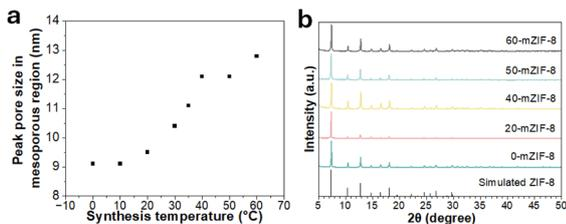
Fig. 2 (a) Synthesis temperature vs. peak pore size in the mesoporous region of *X*-mZIF-8, and (b) XRD spectra of *X*-mZIF-8.
