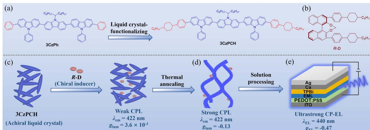
**Scheme 1** (a) Chemical structures of **3CzPh** and liquid crystal-functionalized **3CzPCH**; (b) chemical structure of chiral inducer *R-D*; schematic diagram of the chiral co-assembly process (c) before and (d) after thermal annealing; (e) the device configuration of CP-OLEDs.
