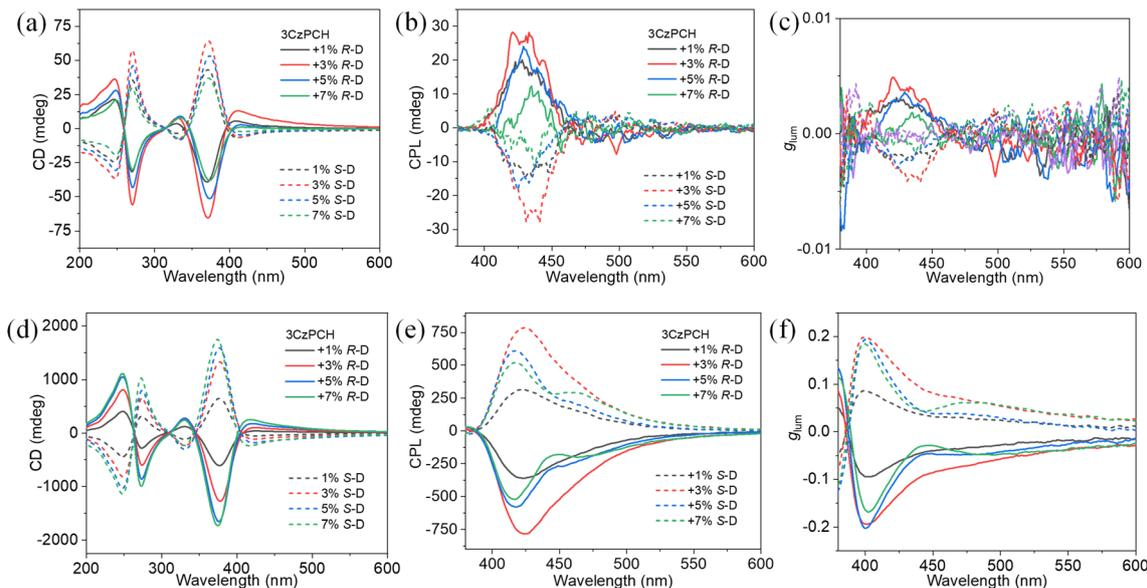
Fig. 3 (a and d) CD spectra, (b and e) CPL spectra, and (c and f)  $g_{lum}$  value curves of **3CzPCH** doped with different wt% amounts of *R/S-D* (a–c: before thermal annealing; d–f: after thermal annealing at 120 °C).
