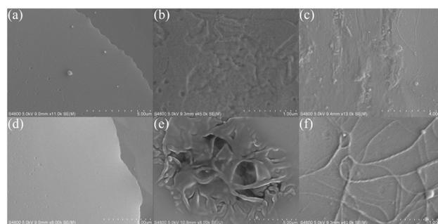
Fig. 4 SEM images of **3CzPCH+3 wt% R-D** (a–c) before and (d–f) after thermal annealing at 120 °C. (a and d)  $10 \text{ mg mL}^{-1}$ , (b and e)  $10^{-1} \text{ mg mL}^{-1}$  and (c and f)  $10^{-3} \text{ mg mL}^{-1}$  in toluene.
