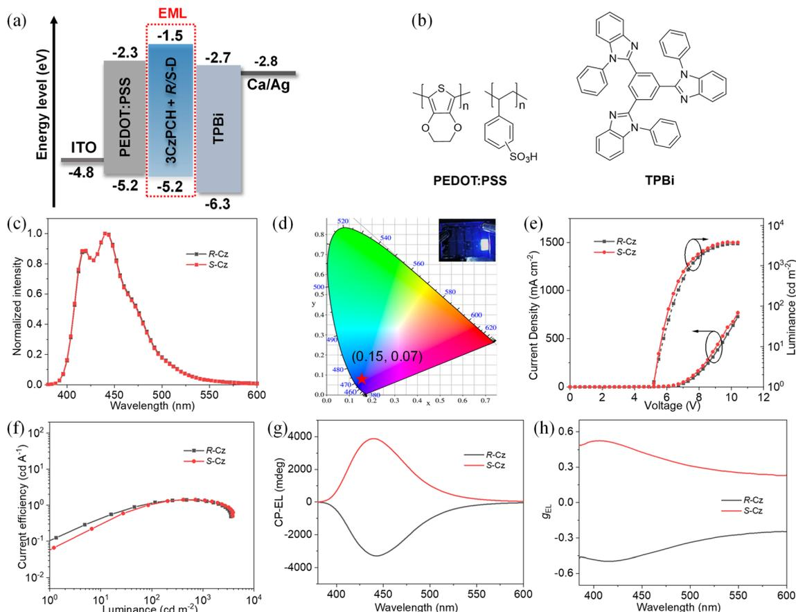
Fig. 5 (a) The energy level diagram of the related materials; (b) chemical structures of functional layer molecules; (c) EL spectra of the *R/S-Cz*; (d) CIE 1931 chromaticity diagram; (e)  $J$ - $V$ - $L$  characteristics; (f) CE- $L$  curves; (g) CP-EL spectra and (h)  $g_{\text{EL}}$  curves of the *R/S-Cz*.
