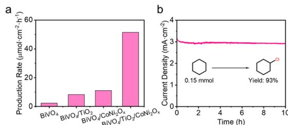
Fig. 3 (a) Production rate of chlorocyclohexane from the C-H chlorination of cyclohexane. Reaction time: 2 h (30 mL NaCl electrolyte, 2 mL cyclohexane, 0.8 V vs. RHE, Ar atmosphere). (b) The J-t curve for the chlorination of 0.15 mmol cyclohexane and the yield of chlorocyclohexane at 0.8 V vs. RHE under an Ar atmosphere. Reaction time: 10 h.
