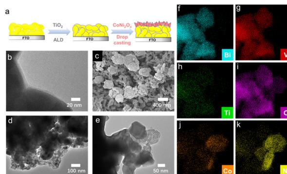
Fig. 1 (a) Schematic illustration of the construction of the  $\text{BiVO}_4/\text{TiO}_2/\text{CoNi}_2\text{O}_x$  photoanode. (b) HRTEM image of  $\text{BiVO}_4/\text{TiO}_2$ . (c) SEM image of  $\text{BiVO}_4/\text{TiO}_2/\text{CoNi}_2\text{O}_x$ . (d and e) HRTEM images of  $\text{BiVO}_4/\text{TiO}_2/\text{CoNi}_2\text{O}_x$ . (f–k) STEM-EDS maps showing the distribution of Bi, V, Ti, O, Co, and Ni in  $\text{BiVO}_4/\text{TiO}_2/\text{CoNi}_2\text{O}_x$ .
