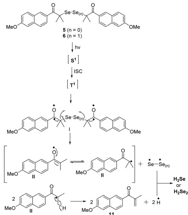
Scheme 11 Proposed mechanism of  $\text{H}_2\text{Se}_2/\text{H}_2\text{Se}$  formation from **5** and **6**.
