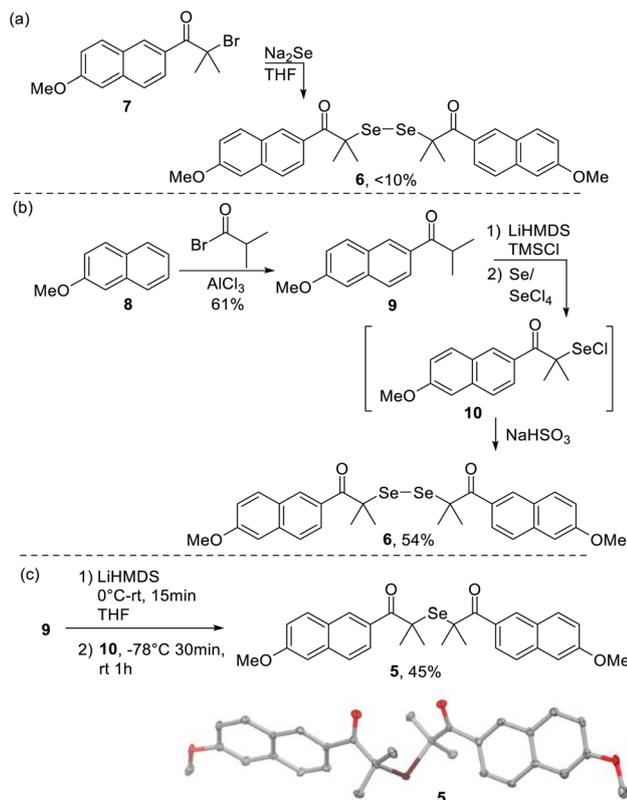
Scheme 7 (A) Reaction of 7 with  $\text{Na}_2\text{Se}$ . (B) Synthesis of naphthacyl-derived diselenide 6. (C) Synthesis of naphthacyl-derived monoselenide 5 and thermal ellipsoid plot of 5 displayed at 50% probability.
