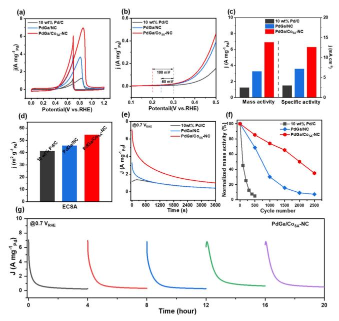
Fig. 3 Catalytic EOR performance measurements. (a) Mass-normalized CV curves, (b) mass-normalized LSV curves, (c) MA and SA, (d) ECSA, (e) CA curves at  $0.7~V_{RHE}$ , (f) ADT tests of PdGa/Co<sub>SA</sub>-NC, PdGa/NC and commercial Pd/C in  $1~M~KOH + 1~M~C_2H_5OH$ , and (g) long-term durability of PdGa/Co<sub>SA</sub>-NC. The catalyst reactivation and electrolyte replacement were done after every 4 hours.
