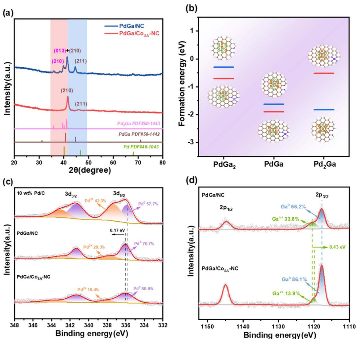
Fig. 2 Structural characterization of the as-prepared catalysts. (a) XRD patterns; (b) formation energies of PdGa<sub>2</sub>, PdGa and Pd<sub>2</sub>Ga on Co<sub>SA</sub>-NC or N-C; (c) Pd 3d XPS spectra; (d) Ga 2p XPS spectra.
