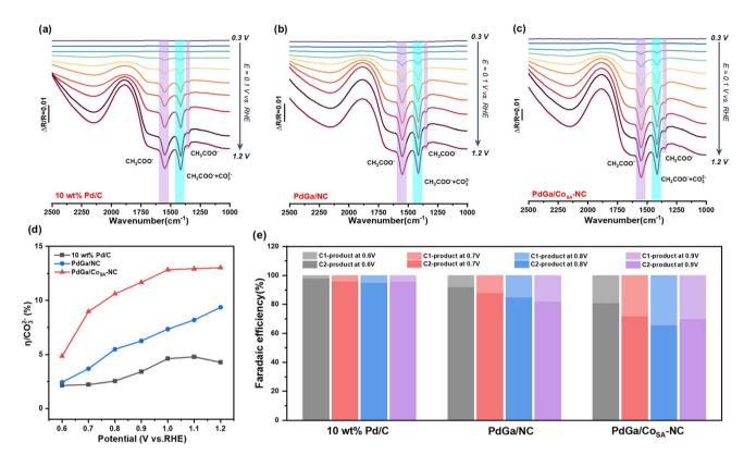
Fig. 4 Electrochemical *in situ* FTIR spectra of (a) commercial Pd/C, (b) PdGa/NC and (c) PdGa/Co<sub>SA</sub>-NC in 1 M KOH + 1 M C<sub>2</sub>H<sub>5</sub>OH; (d) the selectivity ( $\eta$ ) for complete ethanol oxidation to CO<sub>3</sub><sup>2-</sup> from 0.6 to 1.2  $V_{\rm RHE}$ ; (e) the faradaic efficiencies of the C1 pathway and C2 pathway from 0.6 to 0.9  $V_{\rm RHE}$  of catalysts.
