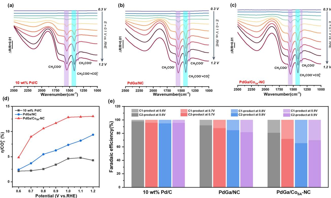
Fig. 4 Electrochemical *in situ* FTIR spectra of (a) commercial Pd/C, (b) PdGa/NC and (c) PdGa/Co<sub>SA</sub>-NC in 1 M KOH + 1 M C<sub>2</sub>H<sub>5</sub>OH; (d) the selectivity ( $\eta$ ) for complete ethanol oxidation to CO<sub>3</sub><sup>2-</sup> from 0.6 to 1.2 V<sub>RHE</sub>; (e) the faradaic efficiencies of the C1 pathway and C2 pathway from 0.6 to 0.9 V<sub>RHE</sub> of catalysts.
