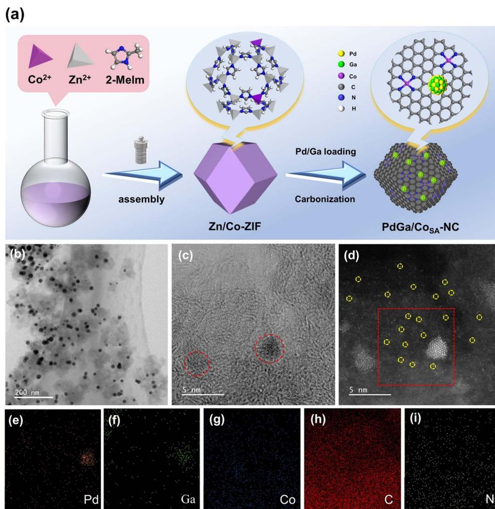
Fig. 1 Synthesis and characterization of PdGa/Co<sub>SA</sub>-NC. (a) Schematic illustration of the synthetic process for PdGa/Co<sub>SA</sub>-NC; (b and c) TEM images of PdGa/Co<sub>SA</sub>-NC; (d–i) HAADF-TEM image and corresponding elemental maps of PdGa/Co<sub>SA</sub>-NC.
