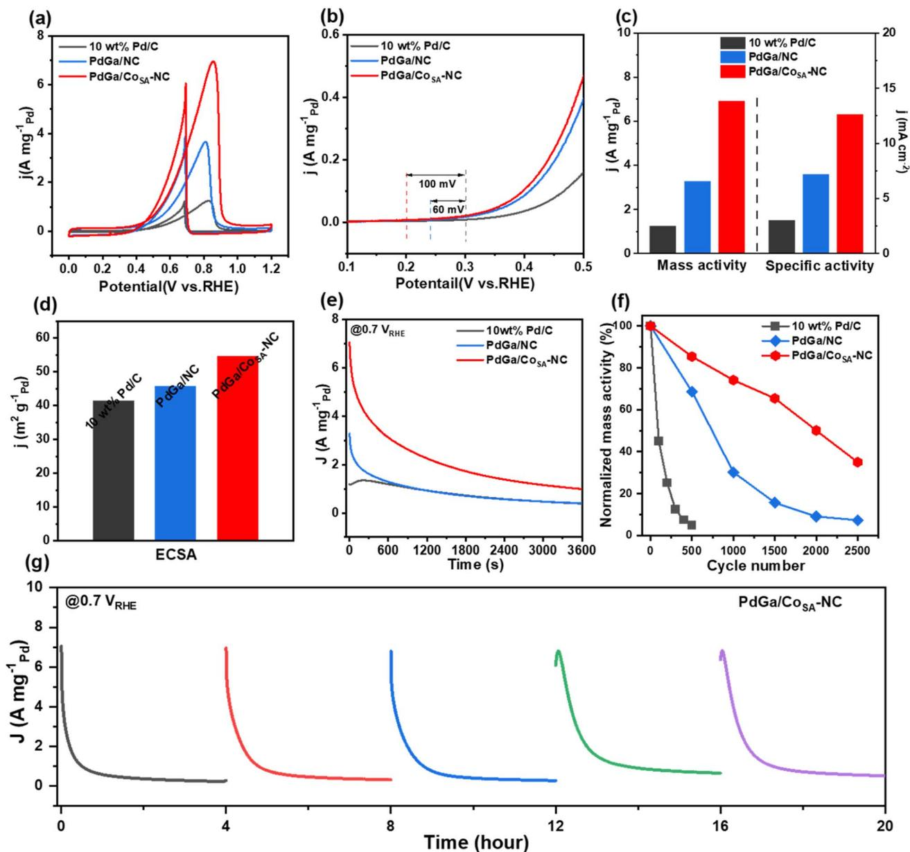
Fig. 3 Catalytic EOR performance measurements. (a) Mass-normalized CV curves, (b) mass-normalized LSV curves, (c) MA and SA, (d) ECSA, (e) CA curves at  $0.7 V_{RHE}$ , (f) ADT tests of PdGa/Co<sub>SA</sub>-NC, PdGa/NC and commercial Pd/C in 1 M KOH + 1 M C<sub>2</sub>H<sub>5</sub>OH, and (g) long-term durability of PdGa/Co<sub>SA</sub>-NC. The catalyst reactivation and electrolyte replacement were done after every 4 hours.
