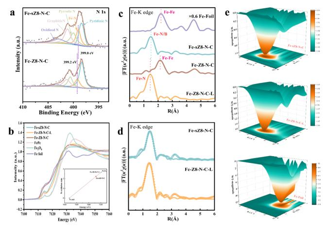
Fig. 2 (a) High-resolution N 1s XPS spectra and (b) Fe K-edge XANES spectra of Fe-sZ8-N-C and other references. (c)  $k^3$ -Weighted Fouriertransformed EXAFS spectra for Fe-sZ8-N-C, Fe-Z8-N-C and the other references. (d) Experimental and best fitting Fe K-edge EXAFS curves for Fe-sZ8-N-C and Fe-Z8-N-C-L in R-space. (e)  $k^3$ -Weighted wavelet transformed Fe K-edge EXAFS spectra of Fe-sZ8-N-C, Fe-Z8-N-C-L and Fe foil.
