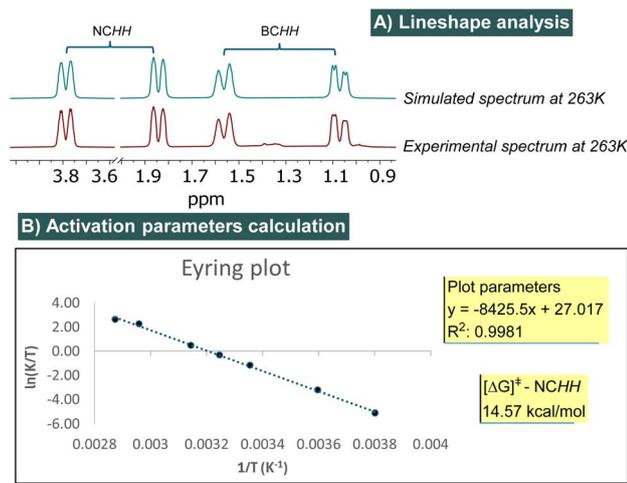
Fig. 2 (A) Simulated  $^1\text{H}$  NMR spectrum obtained from DNMR at  $T = 263$  K with a best overlap fitting obtained at 92.26% vs. the experimental  $^1\text{H}$  NMR spectrum at  $T = 263$  K. (B) Eyring plot obtained for NCHH from DNMR extracted  $k_{\text{ex}}$  values.
