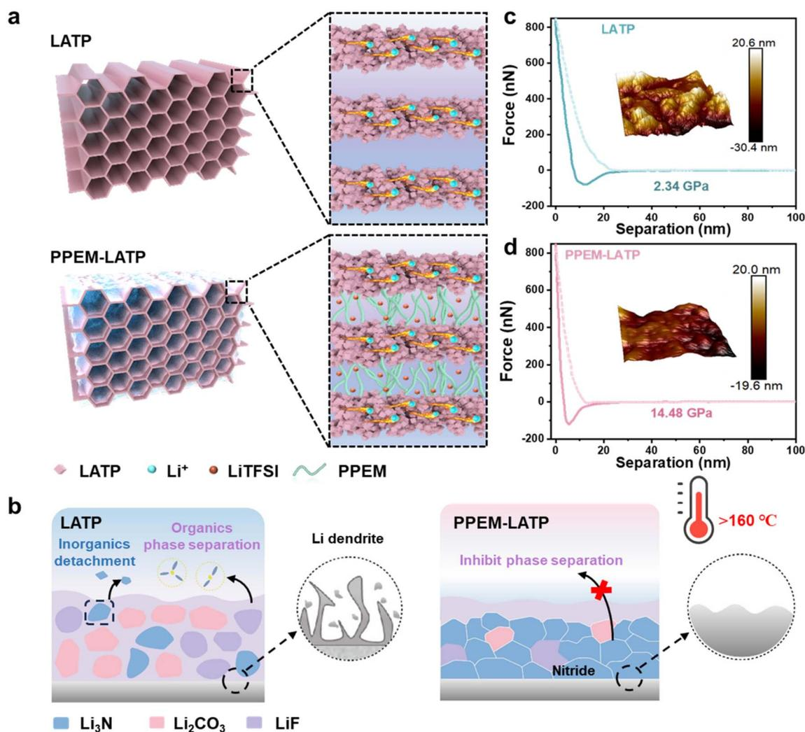
Fig. 4 Characteristics of composite solid-state electrolytes for all-around-safety lithium batteries. (a) Schematic illustration of *in situ* polymerization to prepare the PPEM–LAMP composite solid electrolyte. (b) Diagram of the SEI after cycling of LAMP and PPEM–LAMP in a 160 °C environment. AFM testing of post-cycling: (c) LAMP and (d) PPEM–LAMP lithium anode surface roughness and force–displacement curves.
