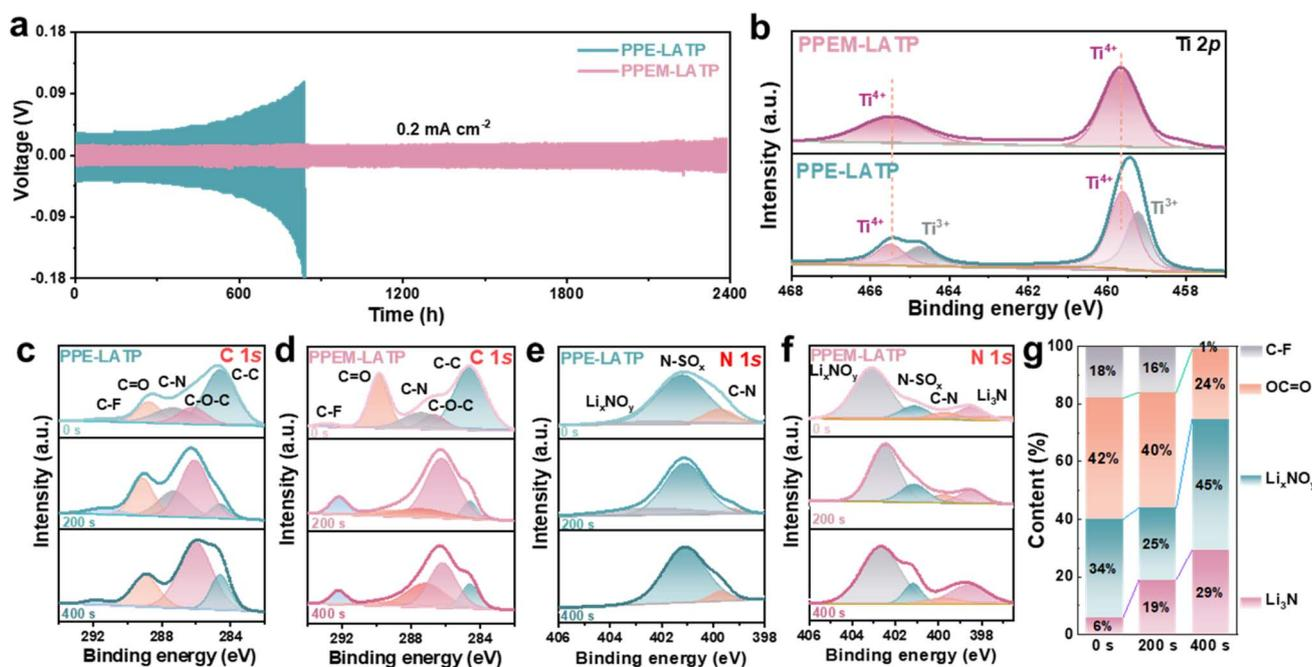
Fig. 3 Anode stability analysis of the PPEM-LATP electrolyte. (a) Li||Li symmetrical battery with PPEM-LATP at a current density of  $0.2\text{ mA cm}^{-2}$ . (b) XPS spectra of Ti 2p in Li||Li cells with PPE-LATP and PPEM-LATP after cycles. (c-f) XPS spectra of C 1s and N 1s in Li||Li cells with PPE-LATP and PPEM-LATP after 10 cycles. (g) Relative contents of C-F, O-C=O and  $\text{Li}_3\text{N}$  in SEI layers at different etching depths.
