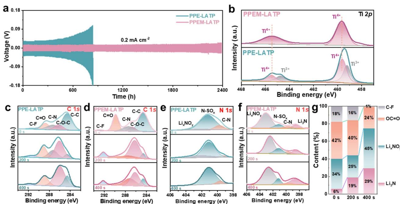
Fig. 3 Anode stability analysis of the PPEM-LATP electrolyte. (a) Li/Li symmetrical battery with PPEM-LATP at a current density of  $0.2\text{ mA cm}^{-2}$ . (b) XPS spectra of Ti 2p in Li/Li cells with PPE-LATP and PPEM-LATP after cycles. (c-f) XPS spectra of C 1s and N 1s in Li/Li cells with PPE-LATP and PPEM-LATP after 10 cycles. (g) Relative contents of C-F, O-C=O and  $\text{Li}_3\text{N}$  in SEI layers at different etching depths.
