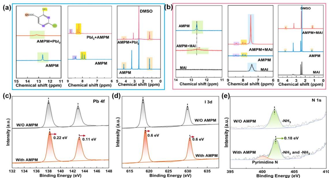
Fig. 2  $^1\text{H}$  NMR spectra of AMPM and AMPM mixed with  $\text{PbI}_2$  (a) and MAI (b) dissolved in  $\text{DMSO}-d_6$  solvent. High-resolution XPS spectra of Pb 4f (c), I 3d (d), and N 1s (e) of original and AMPM-passivated perovskite films.
