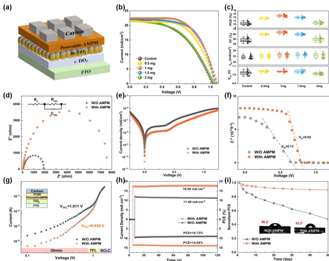
Fig. 5 The device structure (a);  $J-V$  characteristic curves for different additions of AMPM (b). Box plot of parameters of AMPM-treated device at different concentrations (c). EIS curves (d). Dark current (e).  $M-S$  curves (f). SCLC of original and AMPM-treated devices (g). Steady-state output curve (h). Long-term stability test at 30–40% humidity of original and AMPM-passivated C-PSCs. Water contact angle of the original and the AMPM-treated perovskite film (i).
