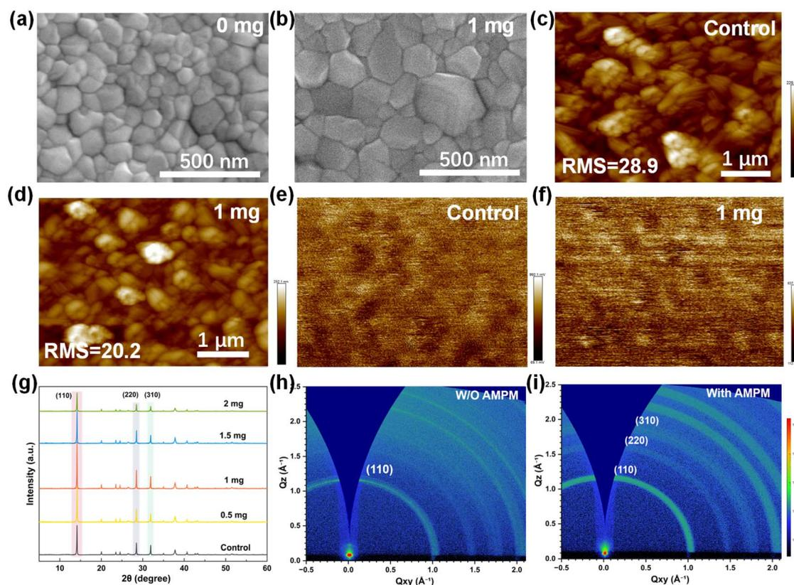
Fig. 3 Top-view SEM images of control perovskite film (a) and perovskite film with  $1\text{ mg}$  AMPM treatment (b). AFM and KPFM images of the control (c and e) and target perovskite films (d and f). XRD patterns of control and  $0.5$ – $2\text{ mg}$  AMPM-treated perovskite films (g). GIWAX patterns for control (h) and  $1\text{ mg}$  AMPM-treated (i) perovskite films.
