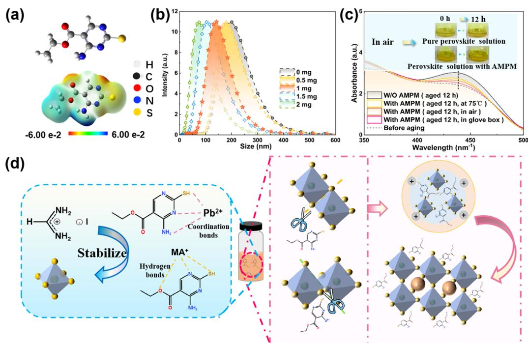
Fig. 1 The molecular structure and ESP of AMPM (a). The colloidal size distributions of control and 0.5–2 mg AMPM-treated perovskite precursor solutions (b). The UV-visible spectra of fresh and 12 h aged perovskite precursor solutions with and without AMPM additive, and images of fresh and 12 h aged perovskite precursor solutions (insets) (c). Schematic diagram showing the mechanism of AMPM's action on perovskite precursors (d).
