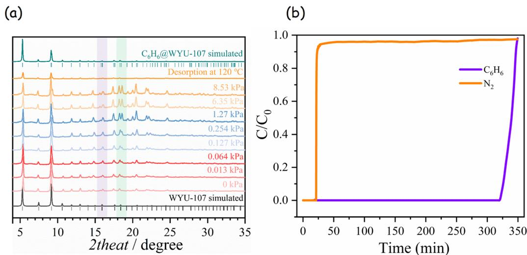
Fig. 3 (a) *In situ* variable-pressure PXRD patterns of WYU-107, collected under benzene vapor pressure from 0 to 8.53 kPa (guest-free to  $C_6H_6@WYU-107$ ) and desorption at 120 °C after the adsorption process. (b) Benzene breakthrough curves for WYU-107 in air at 298 K.
