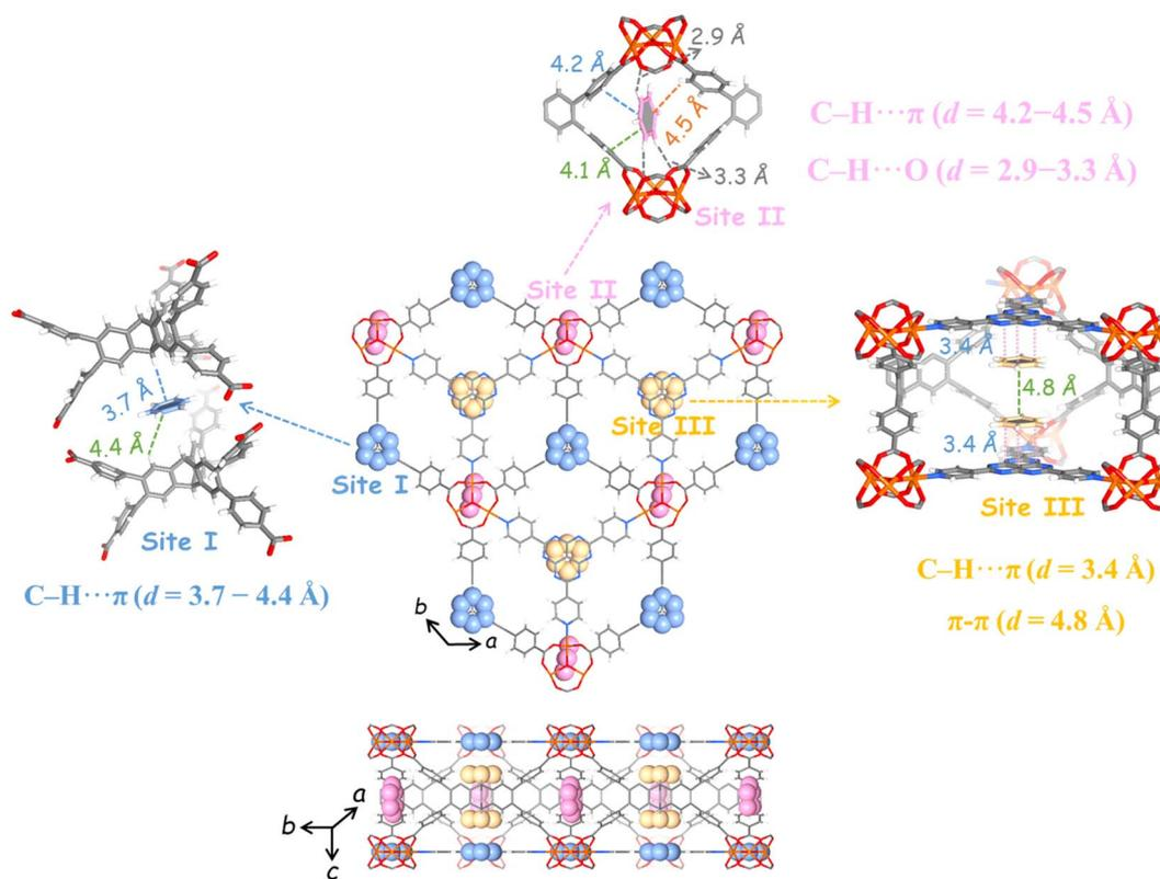
Fig. 4 The adsorption sites of  $C_6H_6@WYU-107$  characterized by single-crystal X-ray diffraction.
