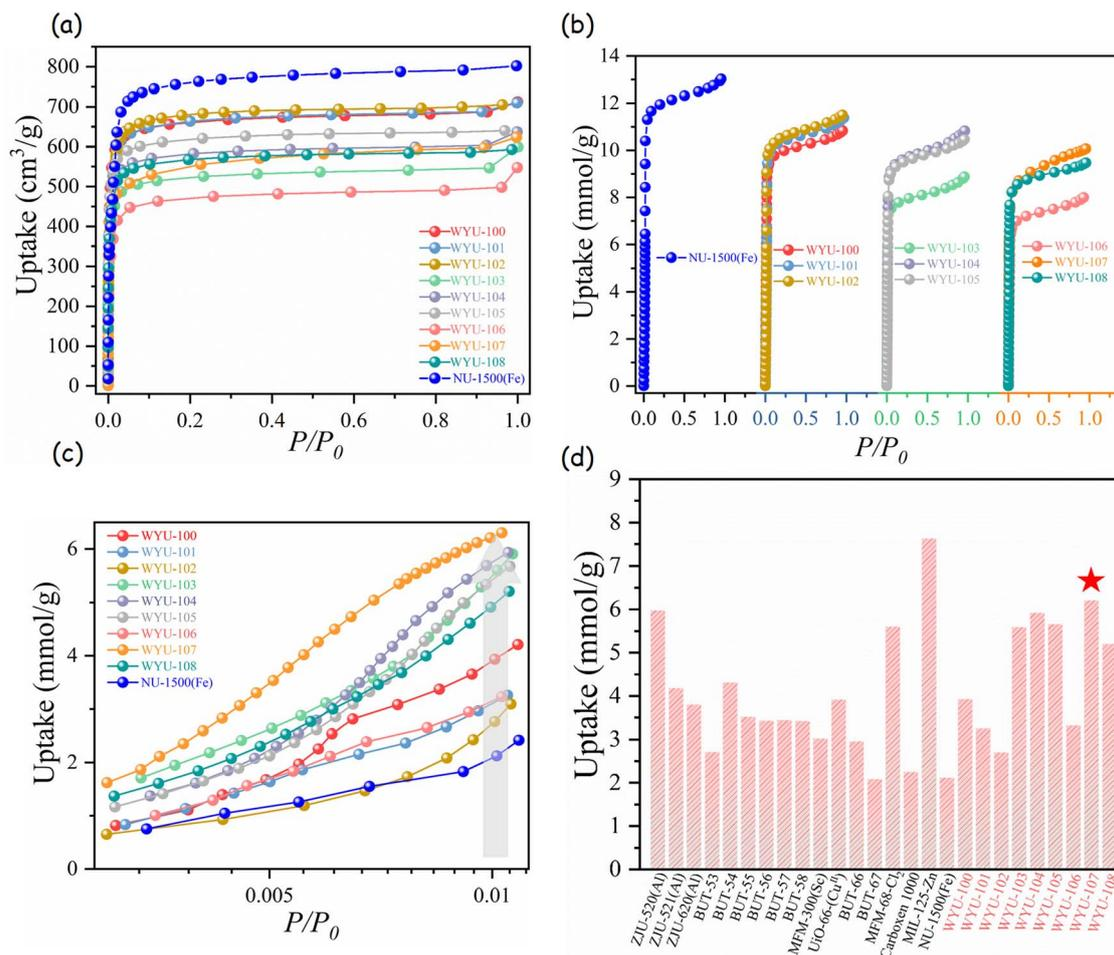
Fig. 2 (a)  $N_2$  sorption isotherms at 77 K and (b) benzene vapor adsorption isotherms at 298 K for **WYU-100–108** and **NU-1500(Fe)**. (c) Logarithmic-scale plots of  $P/P_0 = 0.01$  to view the adsorption of benzene at low partial pressures. (d) The performance comparison of trace benzene vapor uptakes for various MOFs at  $P/P_0 = 0.01$ .
