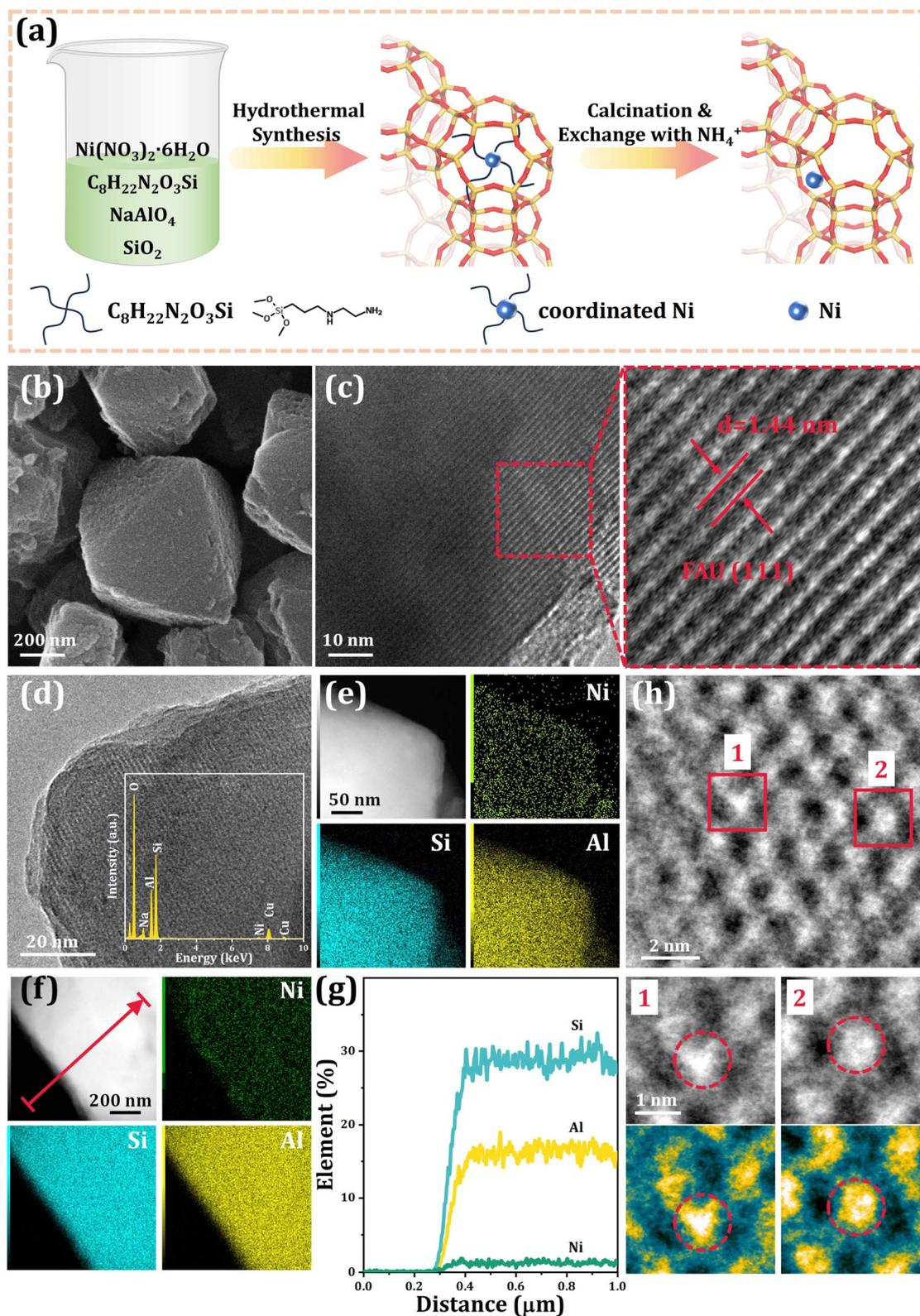
**Fig. 1** Synthesis and characterization of H-Ni@Y. (a) Fabrication process of FAU zeolites and schematic of Ni occupancy in H-Ni@Y; (b) SEM image, (c) HR-TEM and enlarged view of selected region, (d) EDS analysis (the insert was the element dispersive spectrum), (e) EDS mappings, (f and g) line scan (the red arrow indicated the line scan position), and (h) iDPC-STEM images of samples.
