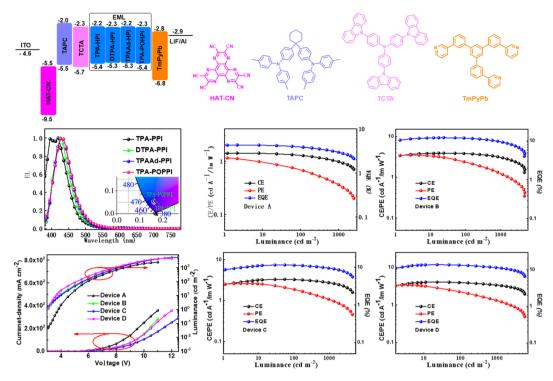
Fig. 5 Energy-level diagram and structure of the devices, chemical structure of the materials used in the OLEDs, voltage-dependent EL spectra of the devices based on TPA-PPI, DTPA-PPI, TPAAd-PPI and TPA-POPPI, current density-voltage-luminance (J-V-L) characteristics and relationship between EL efficiencies and luminance for the devices.
