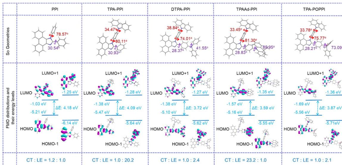
Fig. 2 Molecular geometries in the ground state, FMO distributions and calculated energy levels and the ratio of CT and LE states of PPI, TPA-PPI, DTPA-PPI, TPAAd-PPI and TPA-POPPI.
