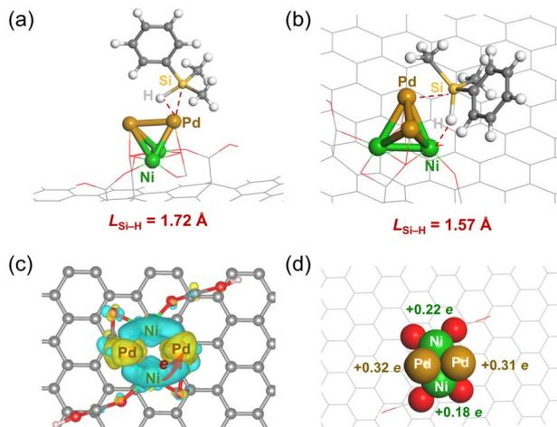
Fig. 5 Optimal structures of PhMe<sub>2</sub>SiH adsorption on PdNi-SLCs/CNTs (a and b). The brown and green atoms represent Pd and Ni atoms, respectively. Differential charge density analysis of PdNi-SLCs/CNTs (c), in which the yellow and cyan colors represent charge accumulation and consumption, respectively, and their isosurface values are all 0.0016 e bohr<sup>-3</sup>. Bader charge analysis of Pd and Ni atoms within PdNi-SLCs/CNTs (d).
