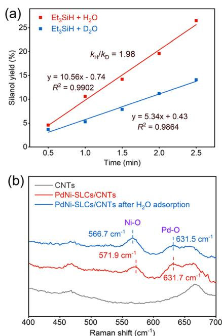
Fig. 6 KIE experiments of dehydrogenative silylation of H<sub>2</sub>O (D<sub>2</sub>O) with Et<sub>3</sub>SiH using PdNi-SLCs/CNTs as the catalyst (a). Raman spectra of PdNi-SLCs/CNTs after adsorption of H<sub>2</sub>O (b).
