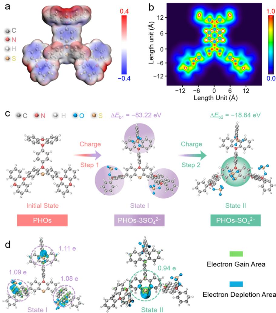
Fig. 4 Theoretical simulations of redox processes of PHOs at various electrochemical states. (a) MEP distribution. (b) ELF- $\pi$  map. (c) Optimized geometries and corresponding  $\Delta E_b$  values after ion coordination. (d) Differential charge isosurfaces at state I and II.
