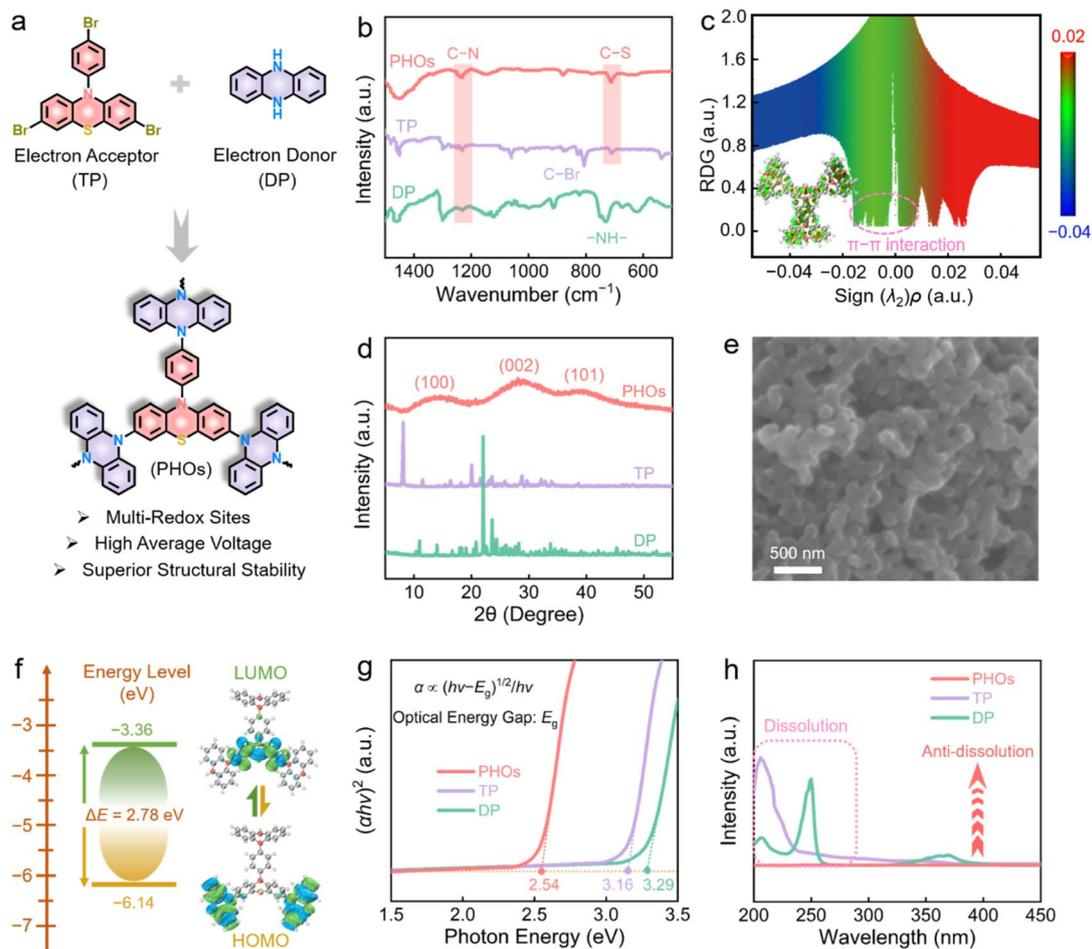
Fig. 1 Structural characterization of PHOs. (a) Synthetic route for PHOs. (b) FT-IR spectra and (c) scatter plots of RDG against  $\text{sign}(\lambda_2)\rho$  and the gradient isosurface. (d) XRD pattern. (e) SEM pattern. (f) Energy levels and frontier molecular orbitals. (g) Calculated  $E_g$  values. (h) UV/Vis spectra of aqueous  $\text{ZnSO}_4$  solution soaked with TP, DP and PHOs for three months.
