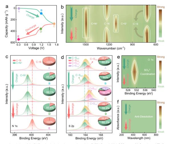
Fig. 5 Structural evolution of the PHO cathode during the operation of the Zn||PHOs cell. (a) A GCD curve. (b) Overview of FT-IR spectra. XPS spectra of (c) N1s, (d) S2p, and (e) O1s at various electrochemical states. (f) UV-vis spectra and photographs of aqueous ZnSO4 electrolyte during (dis)charging.
