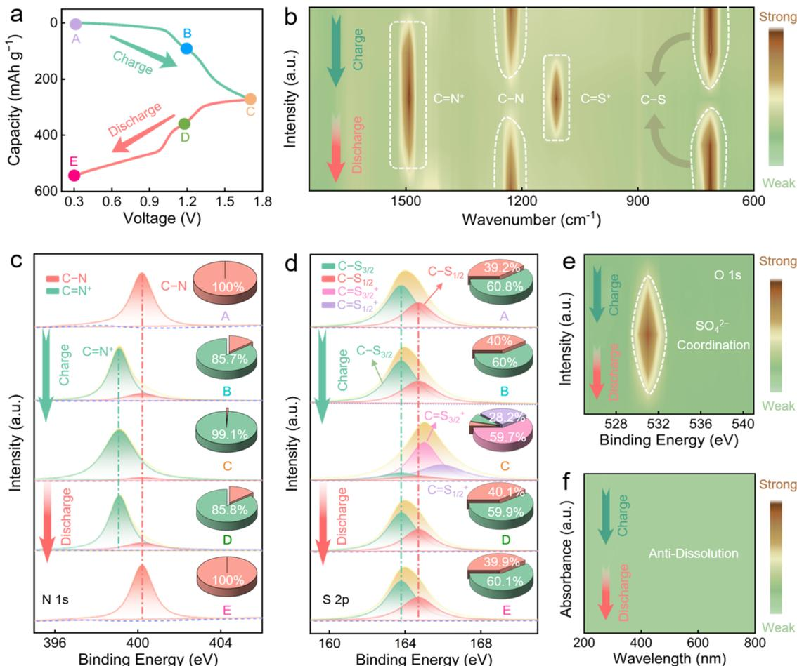
Fig. 5 Structural evolution of the PHO cathode during the operation of the Zn||PHOs cell. (a) A GCD curve. (b) Overview of FT-IR spectra. XPS spectra of (c) N 1s, (d) S 2p, and (e) O 1s at various electrochemical states. (f) UV-vis spectra and photographs of aqueous ZnSO<sub>4</sub> electrolyte during (dis)charging.
