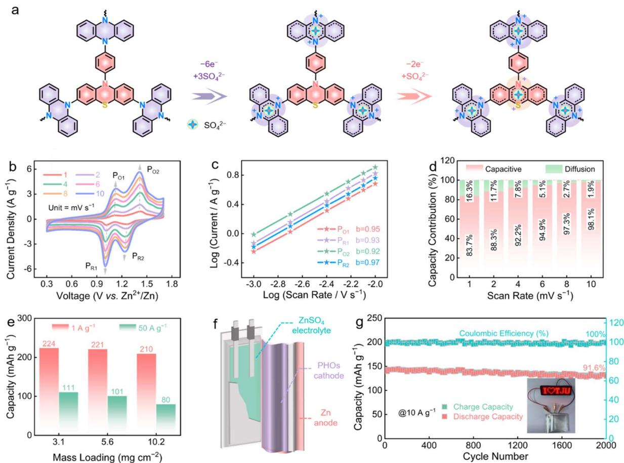
Fig. 6 Charge storage mechanism of the PHO cathode. (a) Two-step bipedal redox behavior of PHOs during the electrochemical charge process. (b) CV curves. (c) Calculated  $b$  values. (d) Capacitive contribution ratios at different scanning rates. (e) Electrochemical performances of the Zn||PHO battery at the practical-level mass. (f) Schematic diagram of a pouch-type Zn||PHO battery. (g) Cycle stability of the pouch battery at a mass loading of  $10.2 \text{ mg cm}^{-2}$  for the PHO cathode.
