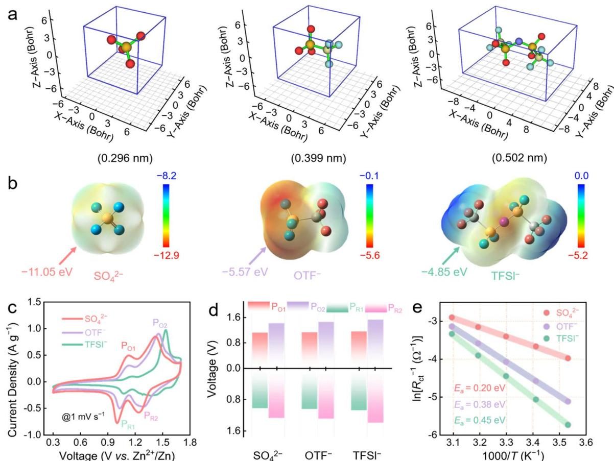
Fig. 2 Electrochemical behavior of PHOs in different electrolytes. (a) Anion size. (b) ESP of the anions. (c) CV curves. (d) Redox peak position. (e) Calculated  $E_a$  values of PHOs in  $\text{SO}_4^{2-}$ ,  $\text{OTF}^-$ , and  $\text{TFSI}^-$  based electrolytes.
