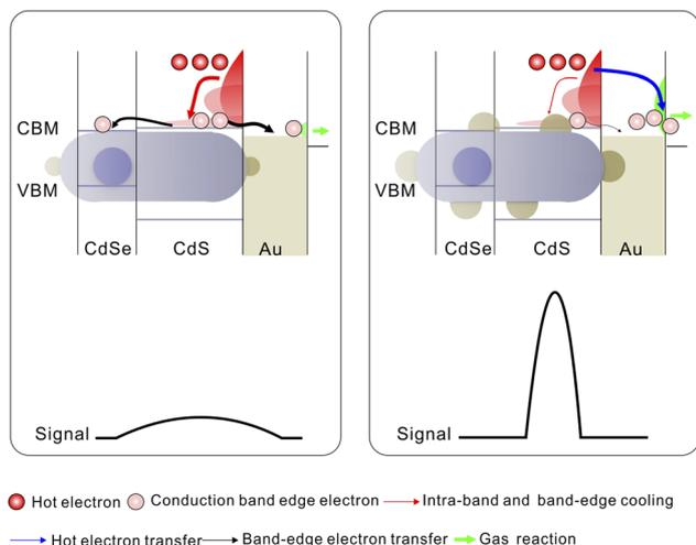
**Scheme 1** Schematic diagram of chemical physical processes for gas-sensing reactivity in CdSe@CdS-Au with two-tip Au domains and CdSe@CdS-Au with large multi-site Au domains and the corresponding detection signal variations. The term response signal refers to the resistance value.
