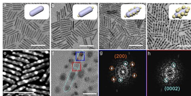
**Fig. 1** Morphological and structural characterization. (a) TEM images of CdSe@CdS. Scale bar, 50 nm. (b) TEM images of CdSe@CdS-TSAu. Scale bar, 50 nm. (c) TEM images of CdSe@CdS-MSAu. Scale bar, 50 nm. (d) TEM images of CdSe@CdS-MBAu. Scale bar, 50 nm. (e) HAADF image of CdSe@CdS-MBAu. Scale bar, 50 nm. (f) High-resolution TEM image of CdSe@CdS-MBAu. Scale bar, 10 nm. (g) The FFT image corresponding to the blue region in (f). (h) The FFT image corresponding to the red region in (f).
