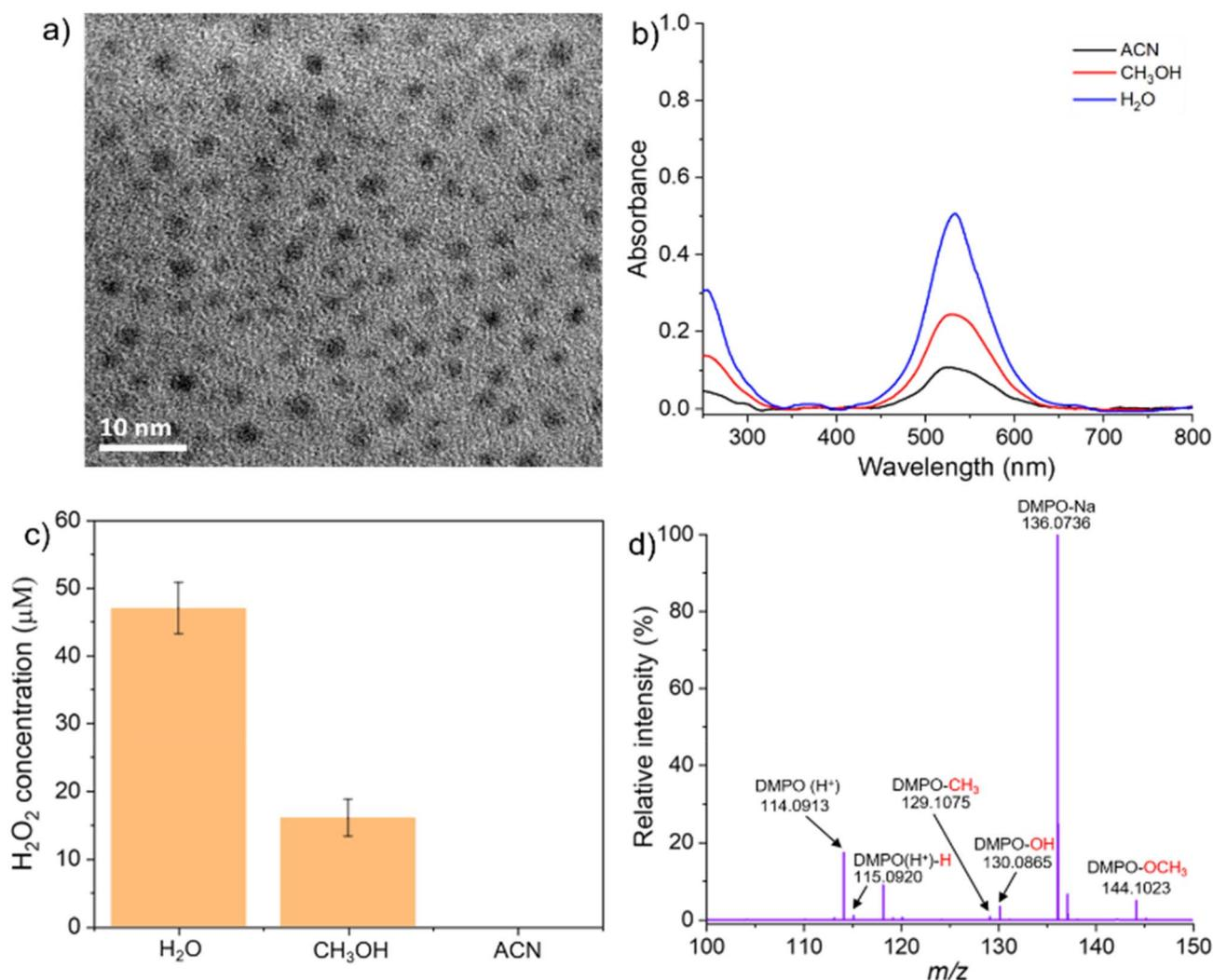
Fig. 5 (a) TEM image of the Au NPs formed when  $CH_3OH$  was used as a solvent. (b) UV-Vis absorption spectra of Au NPs in  $H_2O$ ,  $CH_3OH$ , and ACN solvent. (c) Concentration of  $H_2O_2$  generated using different solvents during the formation of Au NPs. (d) DMPO-based radical capture experiments to confirm the generation of  $\bullet CH_3$  and  $\bullet OCH_3$  during the formation of Au NPs using  $CH_3OH$  as a solvent in microdroplets.
