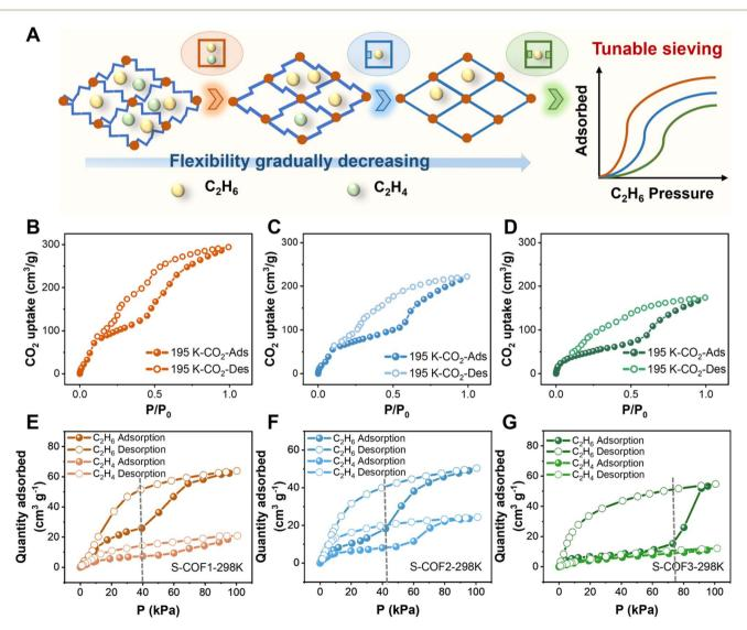
Fig. 3 Investigation of flexible S-COF gas adsorption and separation with the gate-opening mechanism. (A) Schematic diagram of different degrees of flexibility and the gas adsorption separation in flexible S-COF. (B-D) Adsorption isotherms of  $CO_2$  (195 K) for (B) S-COF1, (C) S-COF2 and (D) S-COF3. (E-G)  $C_2H_6$  and  $C_2H_4$  adsorption isotherms of (E) S-COF1, (F) S-COF2 and (G) S-COF3 at 298 K.
