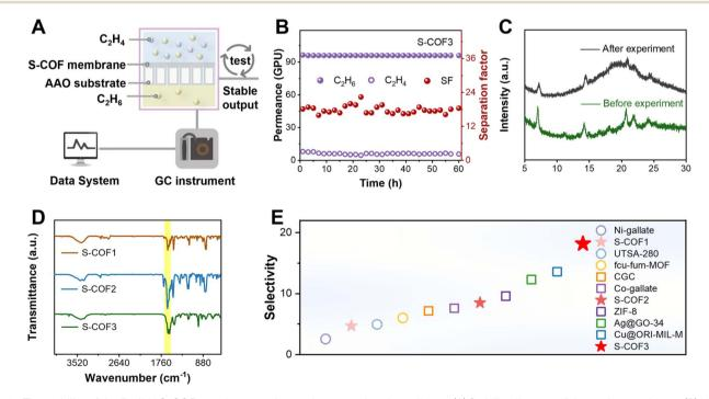
Fig. 5 The stability of the flexible S-COF membrane under varying operational conditions. (A) Stability diagram of the cycle experiment. (B) Longterm separation stability of the S-COF3 membrane. (C) PXRD patterns of the S-COF3 membrane before and after experiments. (D) FT-IR spectra of the S-COF3 membrane after experiments. (E) The comparison of the separation performance between the prepared membranes in this work and other reported membranes in the literature.
