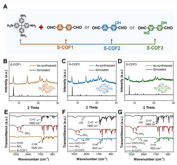
Fig. 1 Synthesis and characterization of S-COFs. (A) Scheme for the preparation of S-COF1, S-COF2 and S-COF3. (B-D) Powder X-ray diffraction patterns of (B) S-COF1, (C) S-COF2, and (D) S-COF3. (E-G) FT-IR spectra of (E) S-COF1, (F) S-COF2, and (G) S-COF3.
