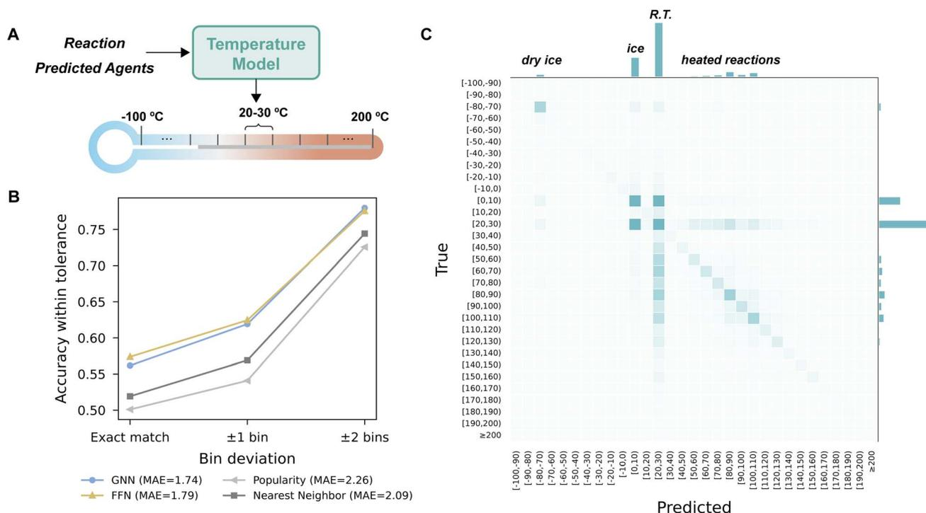
Fig. 4 Individual stage evaluation of temperature prediction. (A) Schematic of the temperature model predicting discrete  $10$  °C bins. (B) Stage 2 temperature prediction accuracy under varying bin tolerances. Bin deviation reflects the distance between the predicted and true bin. The legend reports mean absolute error (MAE) in bin units. (C) Confusion matrix of the best performing FFN model, with the bin distribution for predicted and true values.
