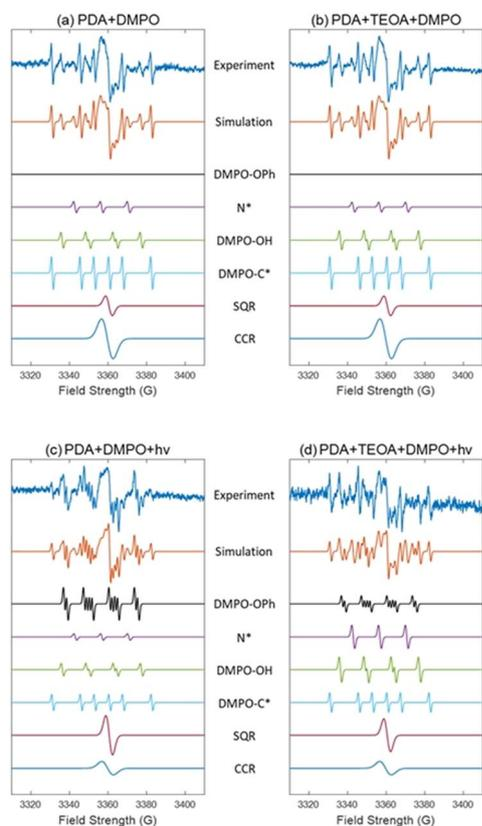
Fig. 6 EPR spectra obtained from aqueous solutions, along with their corresponding numerical simulations, for (a) PDA 60 + DMPO, (b) PDA 60 + TEOA + DMPO, (c) PDA 60 + DMPO +  $h\nu$ , and (d) PDA 60 + TEOA + DMPO +  $h\nu$ . The experimental spectra are the same as in Fig. 5. The simulated spectra are the sum of the individual spectra shown in Table 3.
