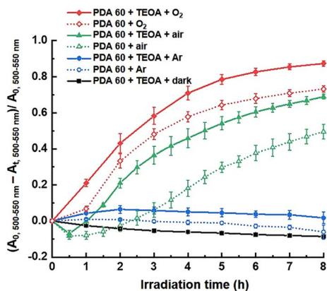
Fig. 8 Photobleaching of PDA 60 under different conditions.
